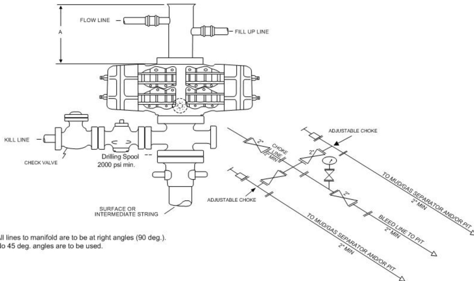
All lines to manifold are to be at right angles (90 deg.).
