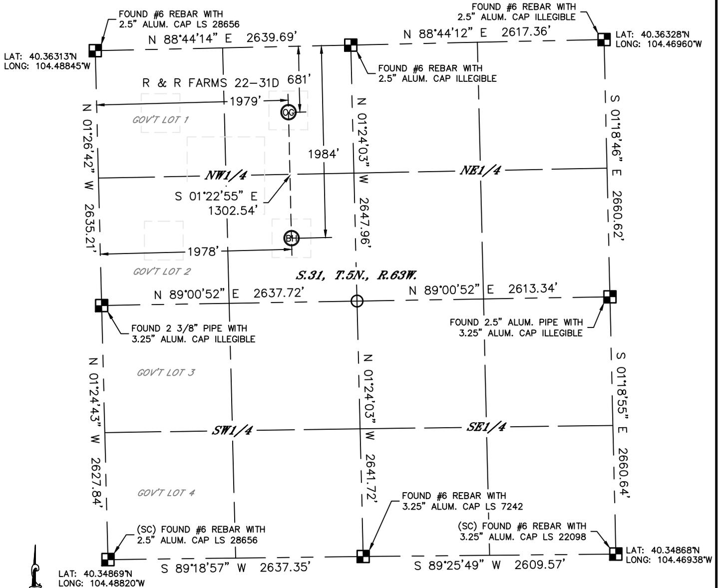
In accordance with a request from Jesse White with APOLLO OPERATING, LLC. Lat40°, Inc. has determined the surface location of the R & R FARMS 22-31D to be 681' from the NORTH line and 1979' from the WEST line and the bottom hole to be 1984' from the NORTH line and 1978' from the WEST line as measured at right angles from the section lines of Section 31, Township 5 North, Range 63 West of the Sixth Principal Meridian, County of Weld, State of Colorado.
