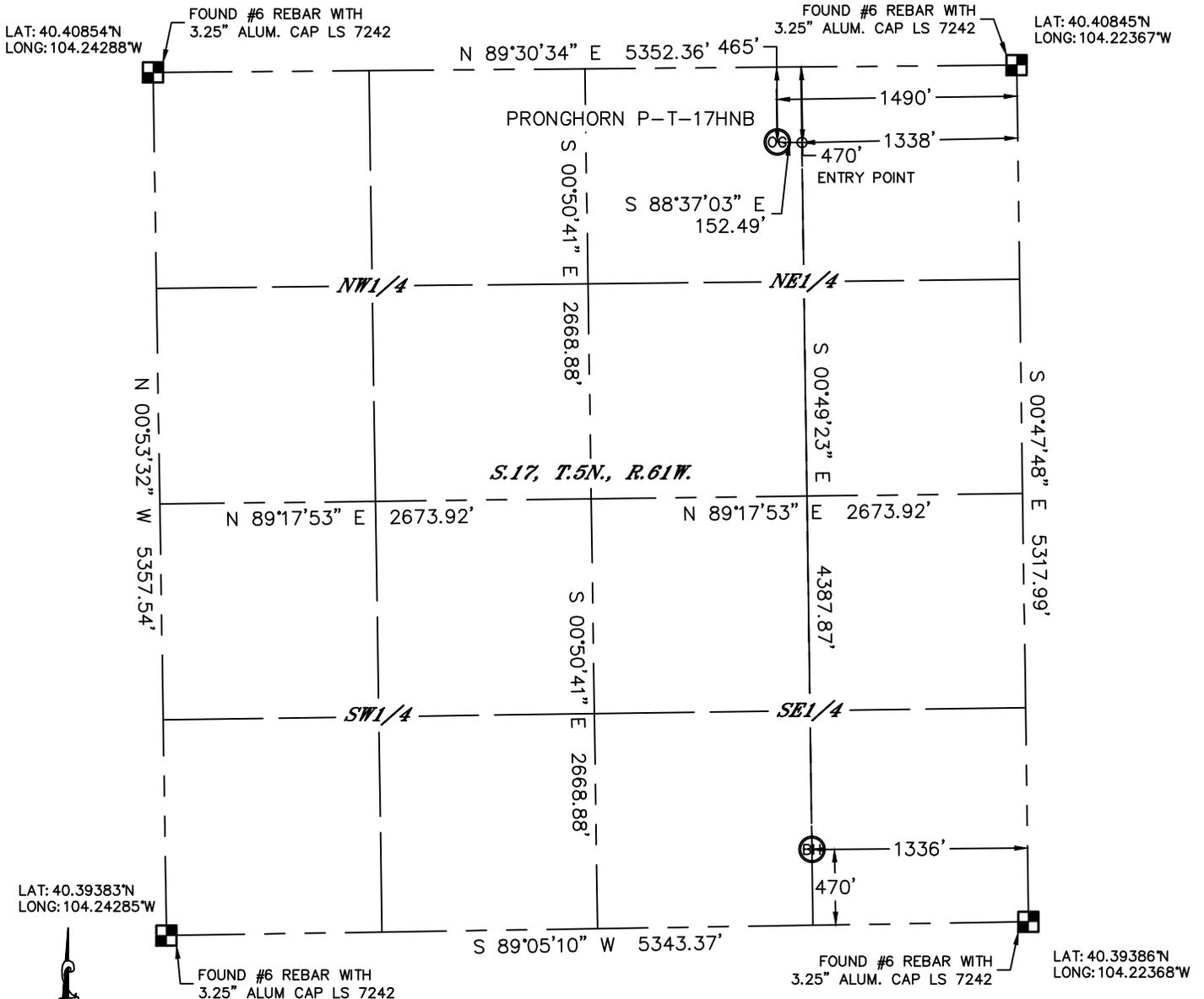
In accordance with a request from Michael Meagher with BONANZA CREEK ENERGY, INC. Lat40°, Inc. has determined the surface location of the PRONGHORN P-T-17HNB to be 465' from the NORTH line and 1490' from the EAST line and the bottom hole to be 470' from the SOUTH line and 1336' from the EAST line as measured at right angles from the section lines of Section 17, Township 5 North, Range 61 West of the Sixth Principal Meridian, County of Weld, State of Colorado.
