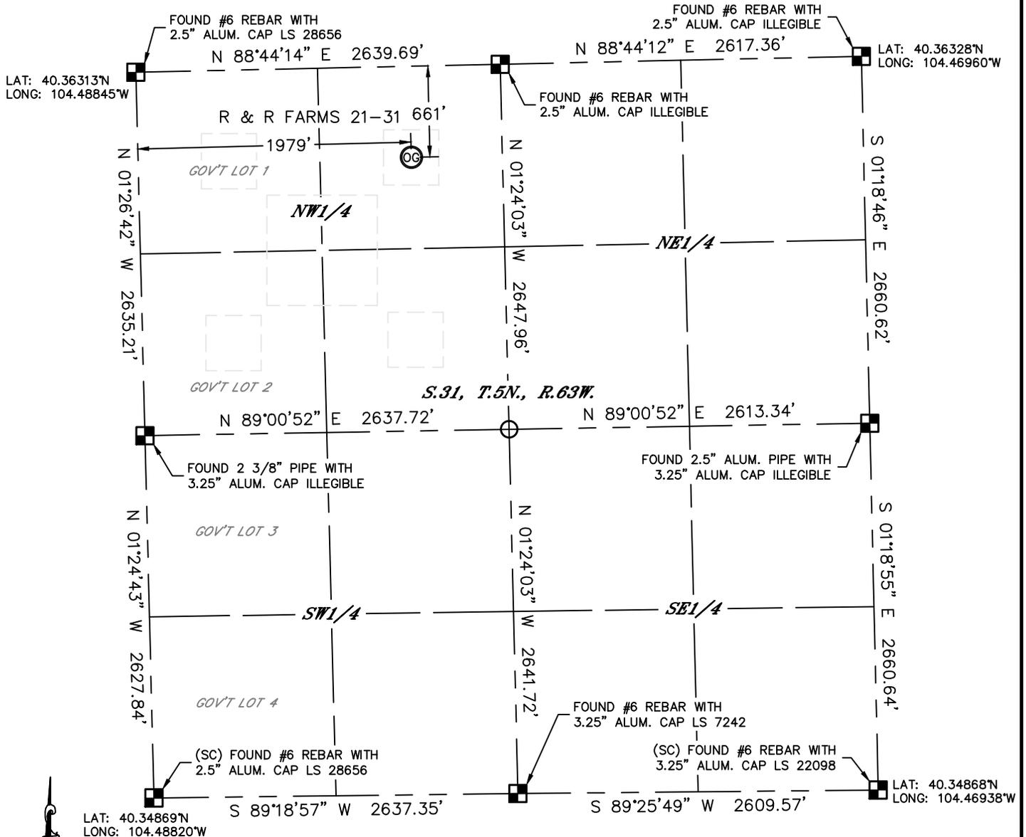
In accordance with a request from Jesse White with APOLLO OPERATING, LLC. Lat40°, Inc. has determined the surface location of the R & R FARMS 21-31 to be 661' from the NORTH line and 1979' from the WEST line as measured at right angles from the section lines of Section 31, Township 5 North, Range 63 West of the Sixth Principal Meridian, County of Weld, State of Colorado.
