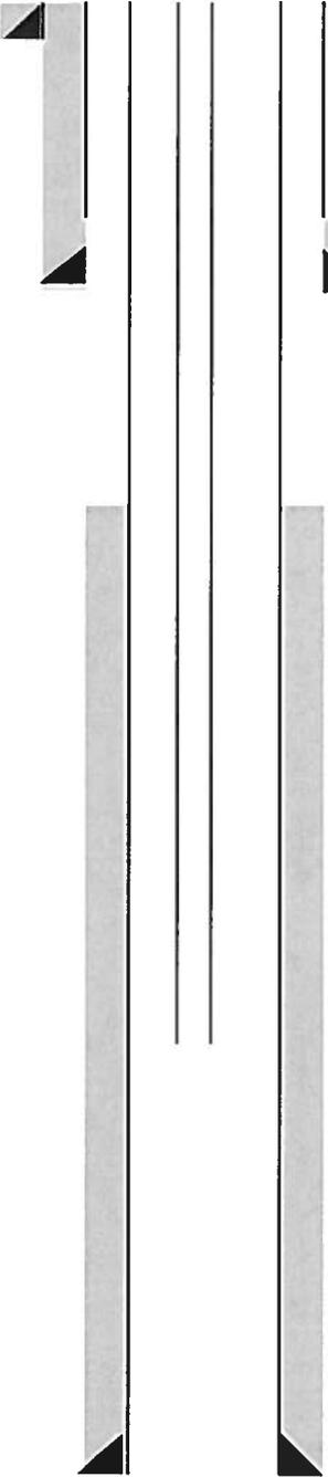
Conductor 24" Hole 16" casing/liner 60' w/44 sks cmt
