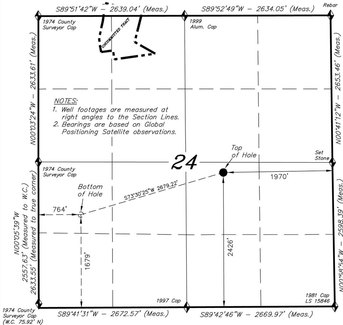
WELL LOCATION, ALP FEE 24-12C (J24), LOCATED AS SHOWN IN THE NW 1/4 SE 1/4 OF SECTION 24, T6S, R93W, 6th P.M. GARFIELD COUNTY, COLORADO.
