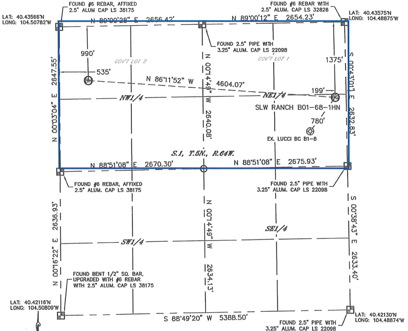
In accordance with a request from Mike Rodine with Noble Energy Inc. Lat40°, Inc. has determined the surface location of the SLW RANCH B01-68-1HN to be 1375' from the NORTH line and 199' from the EAST line and the bottom hole to be 990' from the NORTH line and 535' from the WEST line as measured at right angles from the section lines of Section 1, Township 5 North, Range 64 West of the Sixth Principal Meridian, County of Weld, State of Colorado.
