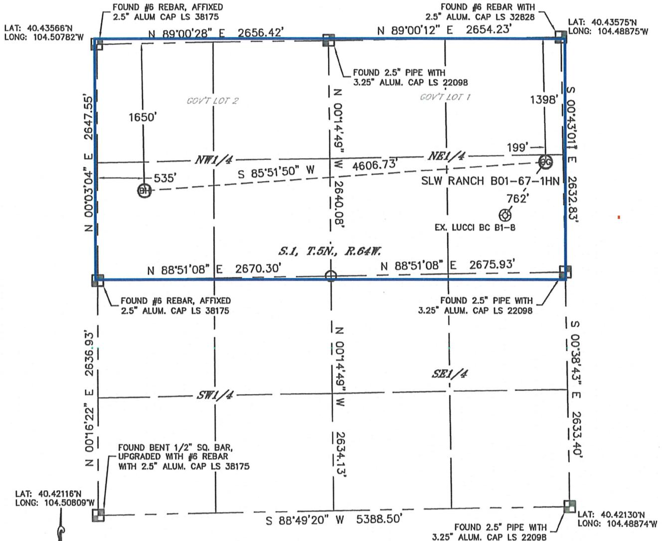
In accordance with a request from Mike Rodine with Noble Energy Inc., Lat40°, Inc. has determined the surface location of the SLW RANCH B01-67-1HN to be 1398' from the NORTH line and 199' from the EAST line and the bottom hole to be 1650' from the NORTH line and 535' from the WEST line as measured at right angles from the section lines of Section 1, Township 5 North, Range 64 West of the Sixth Principal Meridian, County of Weld, State of Colorado.
