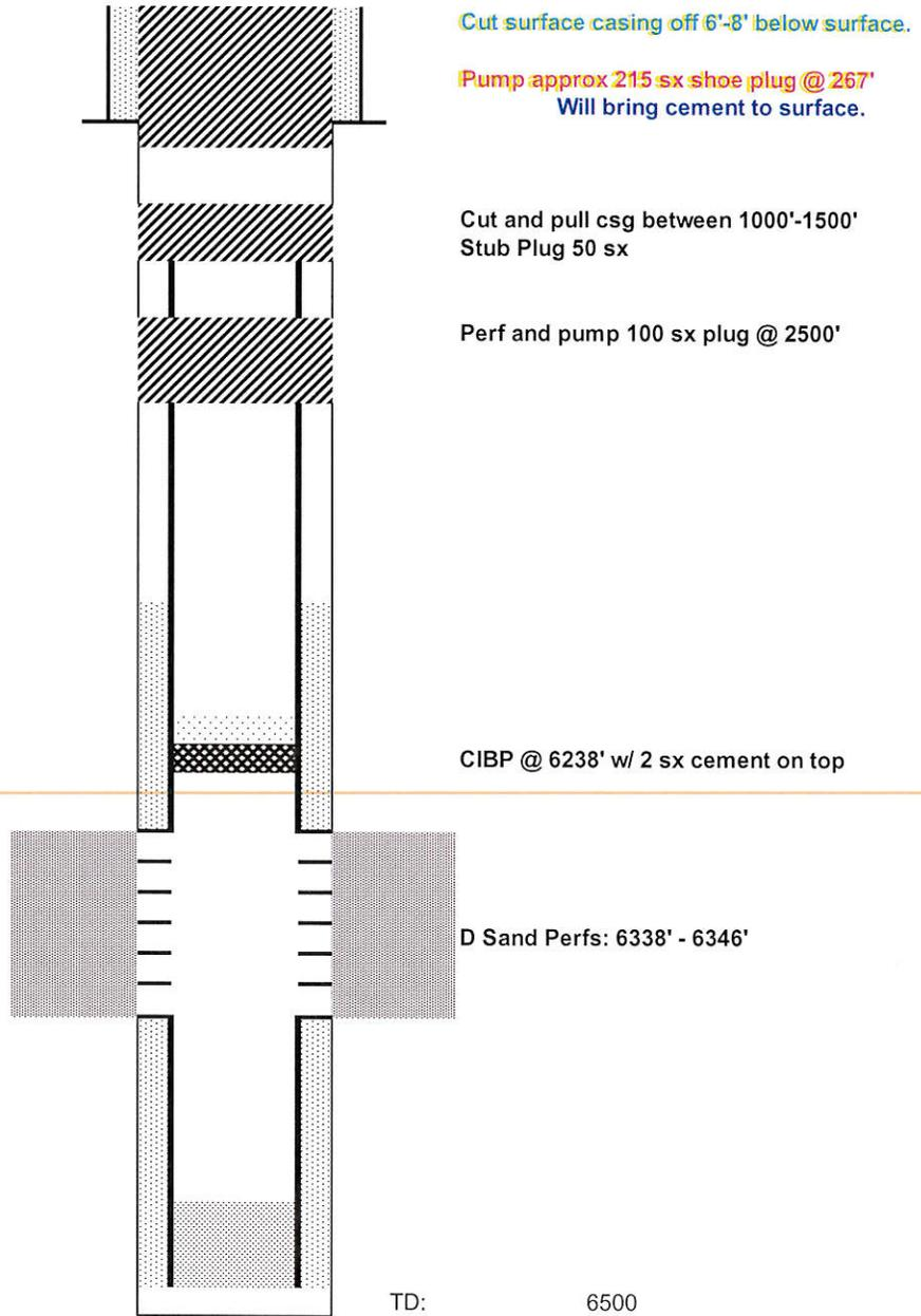
Cut surface casing off 6'-8' below surface.
