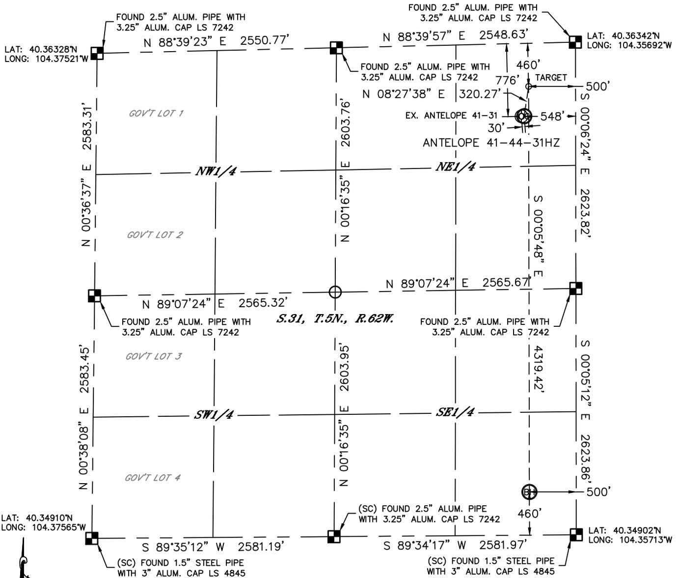
In accordance with a request from Keith Caplan with BONANZA CREEK ENERGY, INC. Lat40°, Inc. has determined the surface location of the ANTELOPE 41-44-31HZ to be 776' from the NORTH line and 548' from the EAST line and the bottom hole to be 460' from the SOUTH line and 500' from the EAST line as measured at right angles from the section lines of Section 31, Township 5 North, Range 62 West of the Sixth Principal Meridian, County of Weld, State of Colorado.
