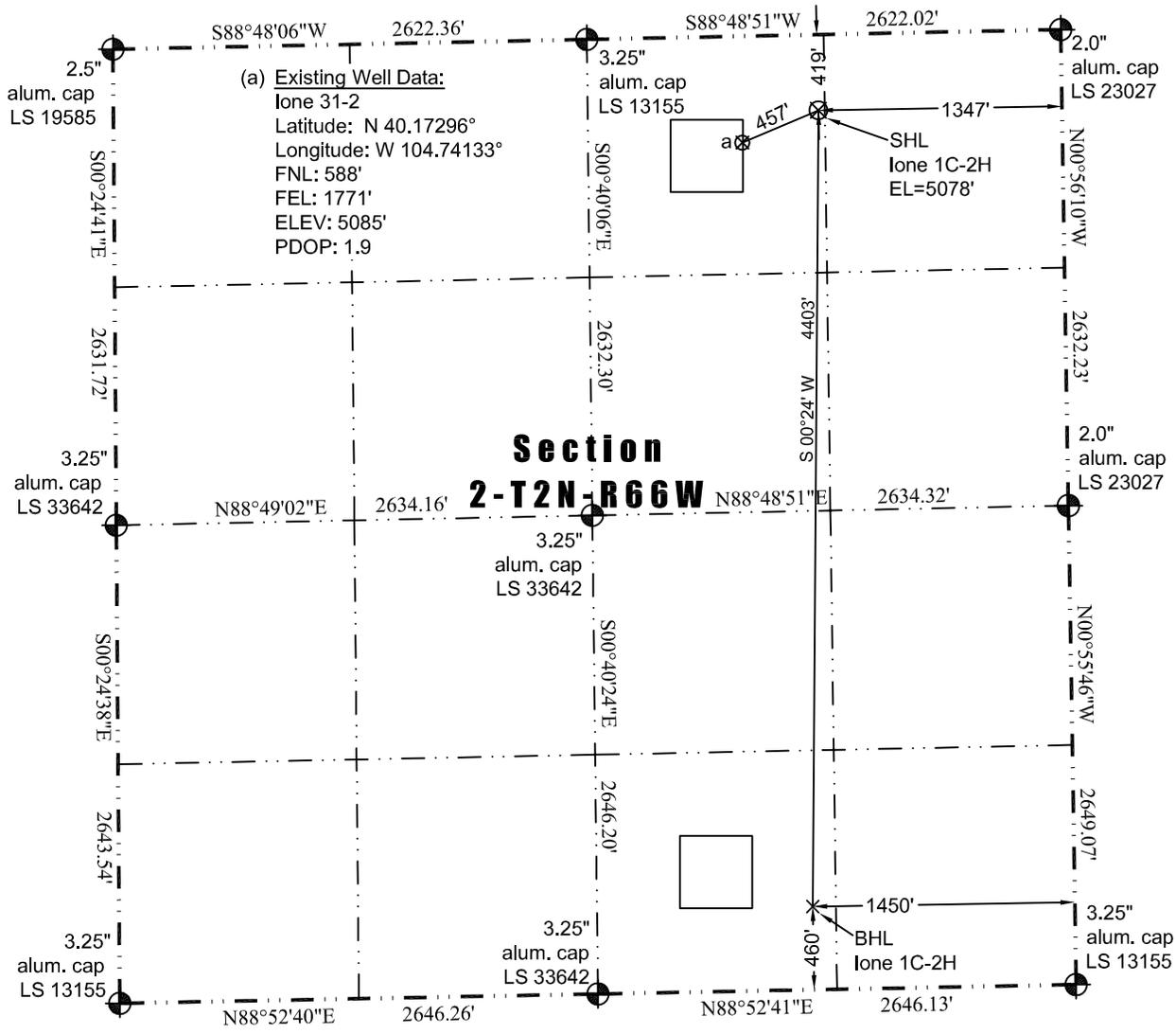
In accordance with a request from Jay Knutson of EnCana Oil & Gas (USA) Inc., JR Land Surveying, LLC has determined the location of the **lone 1C-2H** well site to be SHL 419' FNL and 1347' FEL (BHL 460' FSL and 1450' FEL) as measured at ninety (90) degrees from the section lines of Section 2, Township 2 North, Range 66 West of the 6th Principal Meridian, Weld County, Colorado.
