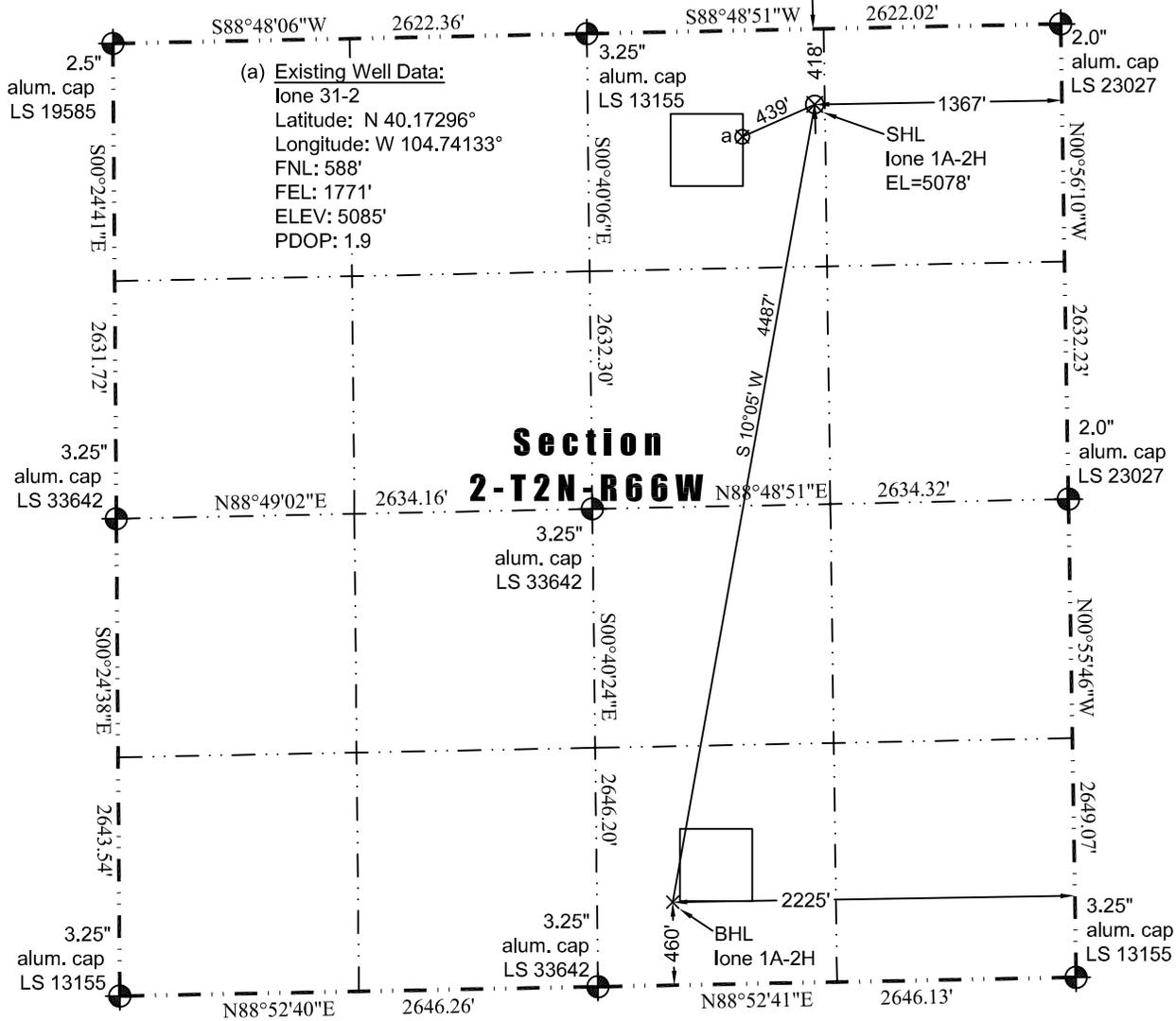
In accordance with a request from Jay Knutson of EnCana Oil & Gas (USA) Inc., JR Land Surveying, LLC has determined the location of the **lone 1A-2H** well site to be SHL 418' FNL and 1367' FEL (BHL 460' FSL and 2225' FEL) as measured at ninety (90) degrees from the section lines of Section 2, Township 2 North, Range 66 West of the 6th Principal Meridian, Weld County, Colorado.
