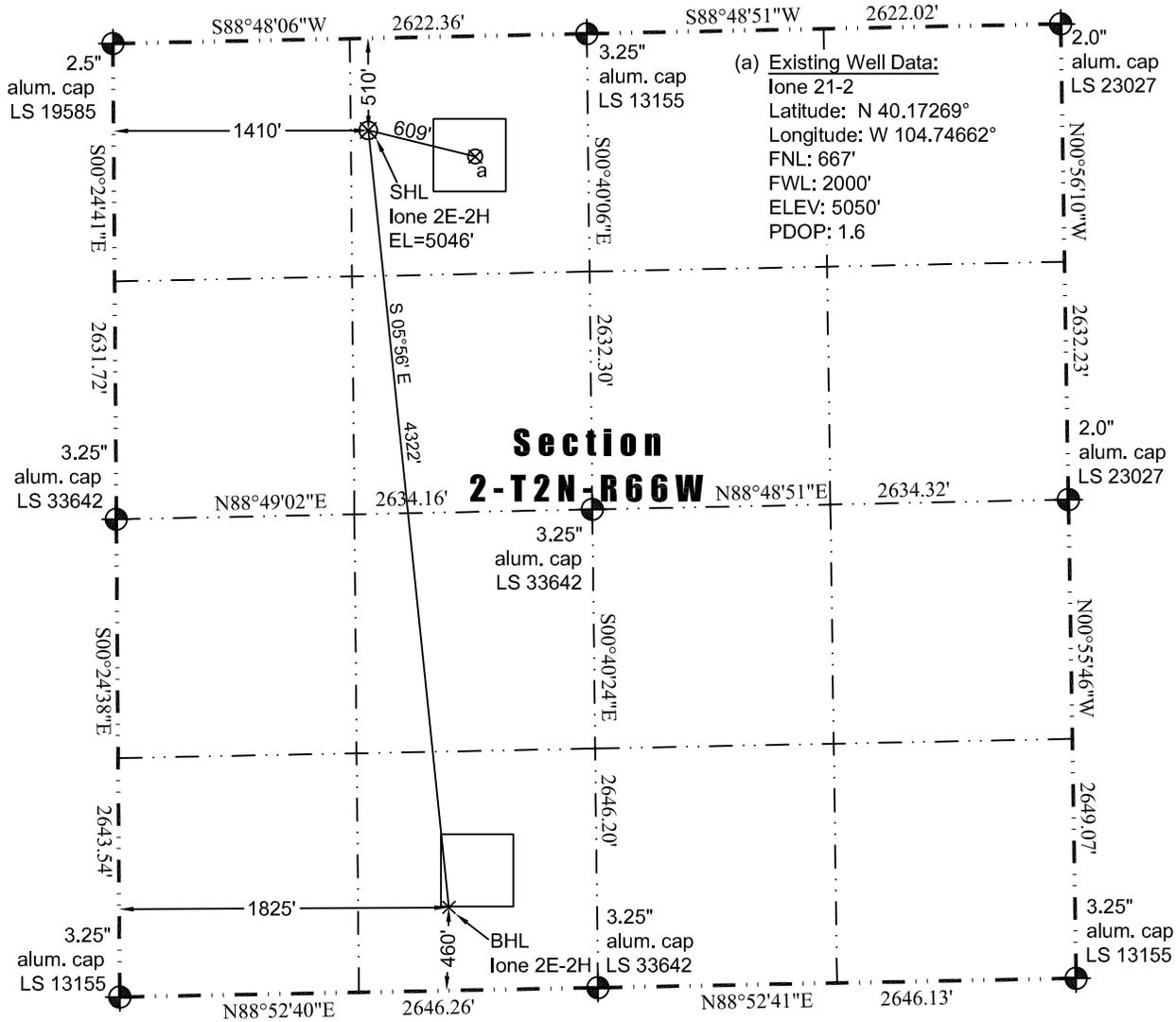
In accordance with a request from Jay Knutson of EnCana Oil & Gas (USA) Inc., JR Land Surveying, LLC has determined the location of the **lone 2E-2H** well site to be SHL 510' FNL and 1410' FWL (BHL 460' FSL and 1825' FWL) as measured at ninety (90) degrees from the section lines of Section 2, Township 2 North, Range 66 West of the 6th Principal Meridian, Weld County, Colorado.
