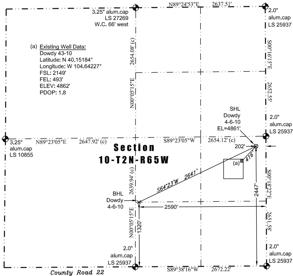
In accordance with a request from Jay Knutson of EnCana Oil & Gas (USA) Inc., JR Land Surveying, LLC has determined the location of the **Dowdy 4-6-10** well site to be SHL: 2447' FSL and 202' FEL, (BHL 1320' FSL and 2590' FEL), as measured at ninety (90) degrees from the section lines of Section 10, Township 2 North, Range 65 West of the 6th Principal Meridian, Weld County Colorado.
