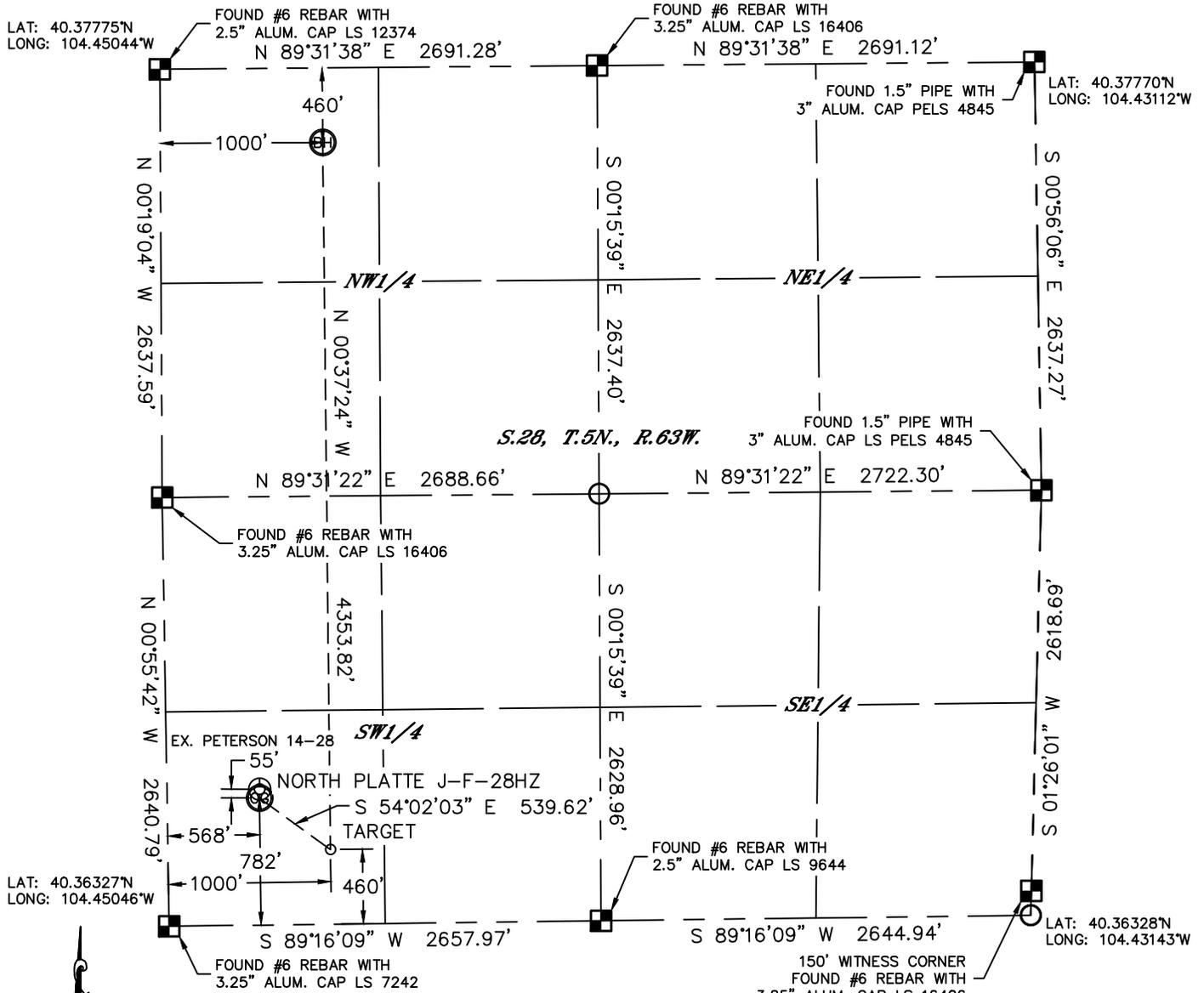
In accordance with a request from Keith Caplan with BONANZA CREEK ENERGY, INC. Lat40°, Inc. has determined the surface location of the NORTH PLATTE J-F-28HZ to be 782' from the SOUTH line and 568' from the WEST line and the bottom hole to be 460' from the NORTH line and 1000' from the WEST line as measured at right angles from the section lines of Section 28, Township 5 North, Range 63 West of the Sixth Principal Meridian, County of Weld, State of Colorado.
