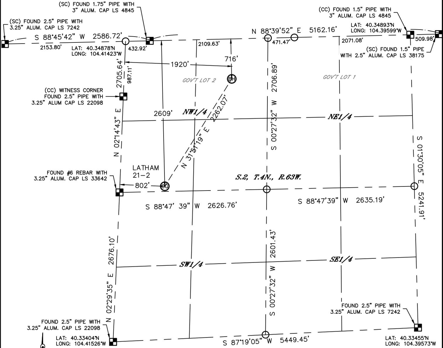
In accordance with a request from Keith Caplan with BONANZA CREEK ENERGY, INC. Lat40°, Inc. has determined the surface location of the LATHAM 21-2 to be 2609' from the NORTH line and 802' from the WEST line and the bottom hole to be 716' from the NORTH line and 1920' from the WEST line as measured at right angles from the section lines of Section 2, Township 4 North, Range 63 West of the Sixth Principal Meridian, County of Weld, State of Colorado.
