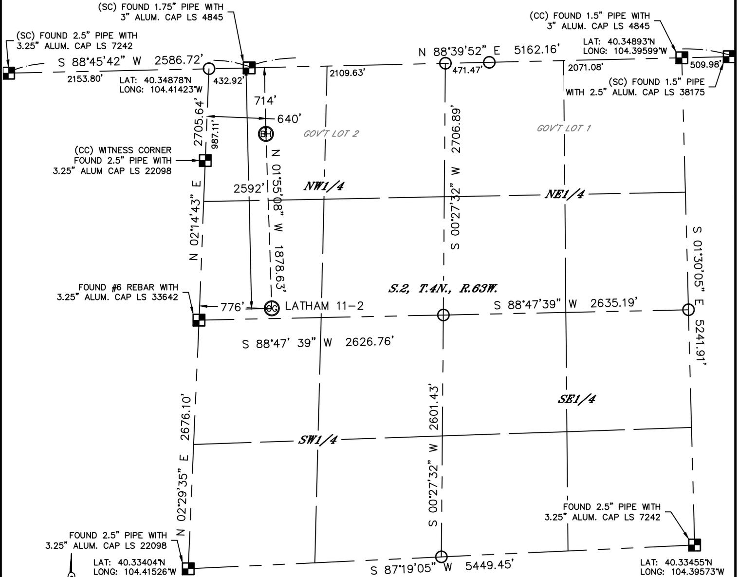
In accordance with a request from Keith Caplan with BONANZA CREEK ENERGY, INC. Lat40°, Inc. has determined the surface location of the LATHAM 11-2 to be 2592' from the NORTH line and 776' from the WEST line and the bottom hole to be 714' from the NORTH line and 640' from the WEST line as measured at right angles from the section lines of Section 2, Township 4 North, Range 63 West of the Sixth Principal Meridian, County of Weld, State of Colorado.
