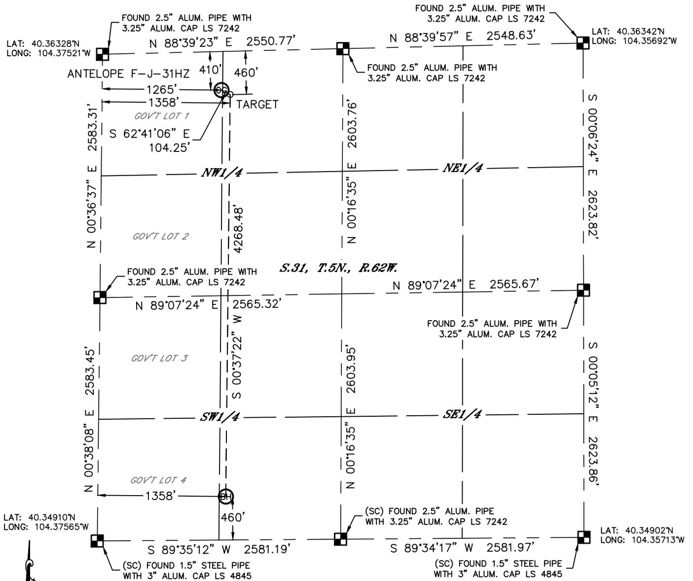
In accordance with a request from Kieth Caplan with BONANZA CREEK ENERGY, INC. Lat40°, Inc. has determined the surface location of the ANTELOPE F-J-31HZ to be 410' from the NORTH line and 1265' from the WEST line and the bottom hole to be 460' from the SOUTH line and 1358' from the WEST line as measured at right angles from the section lines of Section 31, Township 5 North, Range 62 West of the Sixth Principal Meridian, County of Weld, State of Colorado.
