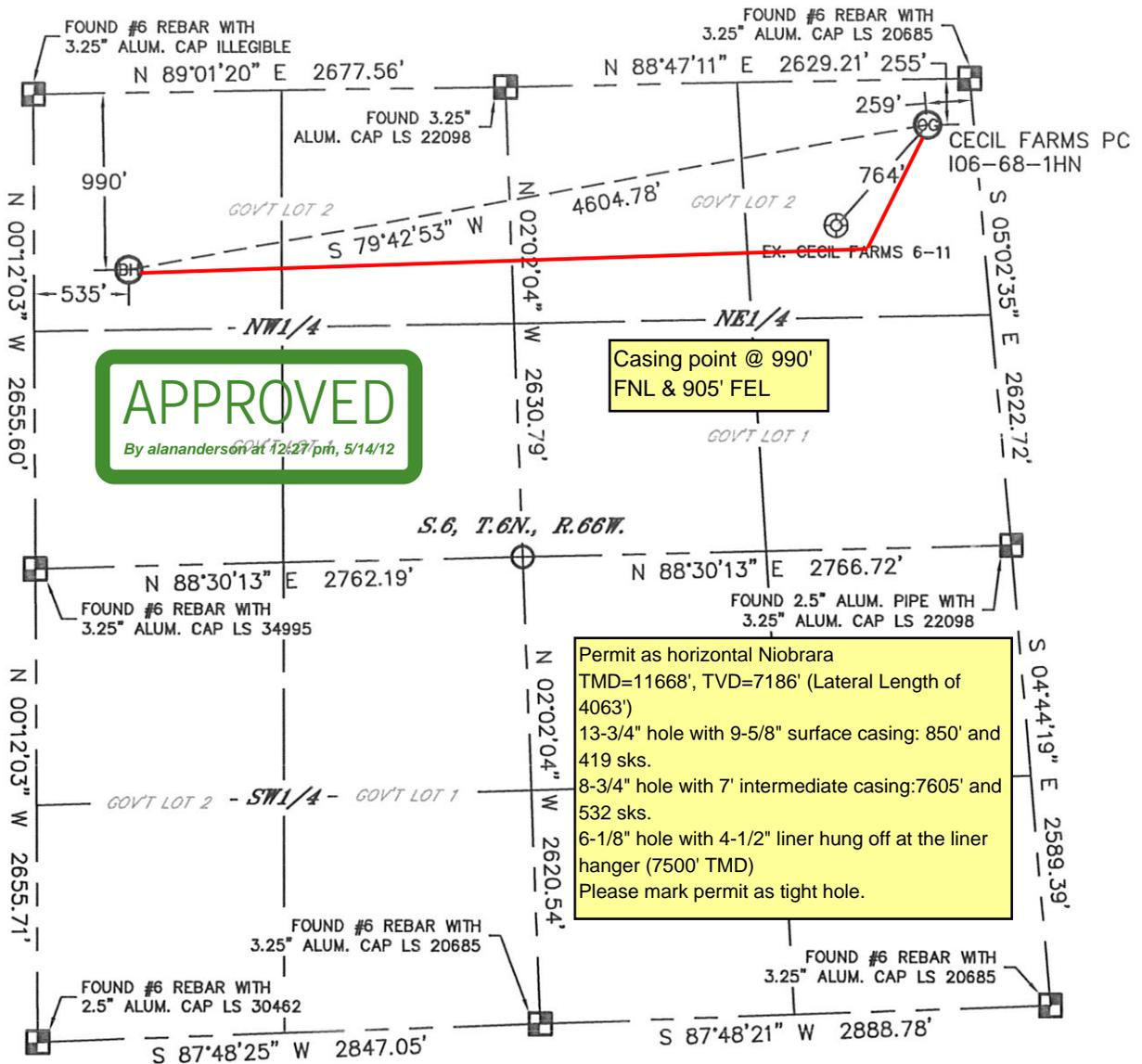
In accordance with a request from Jacob Rice with Noble Energy Inc. Lat40°, Inc. has determined the surface location of the CECIL FARMS PC 106-68-1HN to be 255' from the NORTH line and 259' from the EAST line and the bottom hole to be 990' from the NORTH line and 535' from the WEST line as measured at right angles from the section lines of Section 6, Township 6 North, Range 66 West of the Sixth Principal Meridian, County of Weld, State of Colorado.
