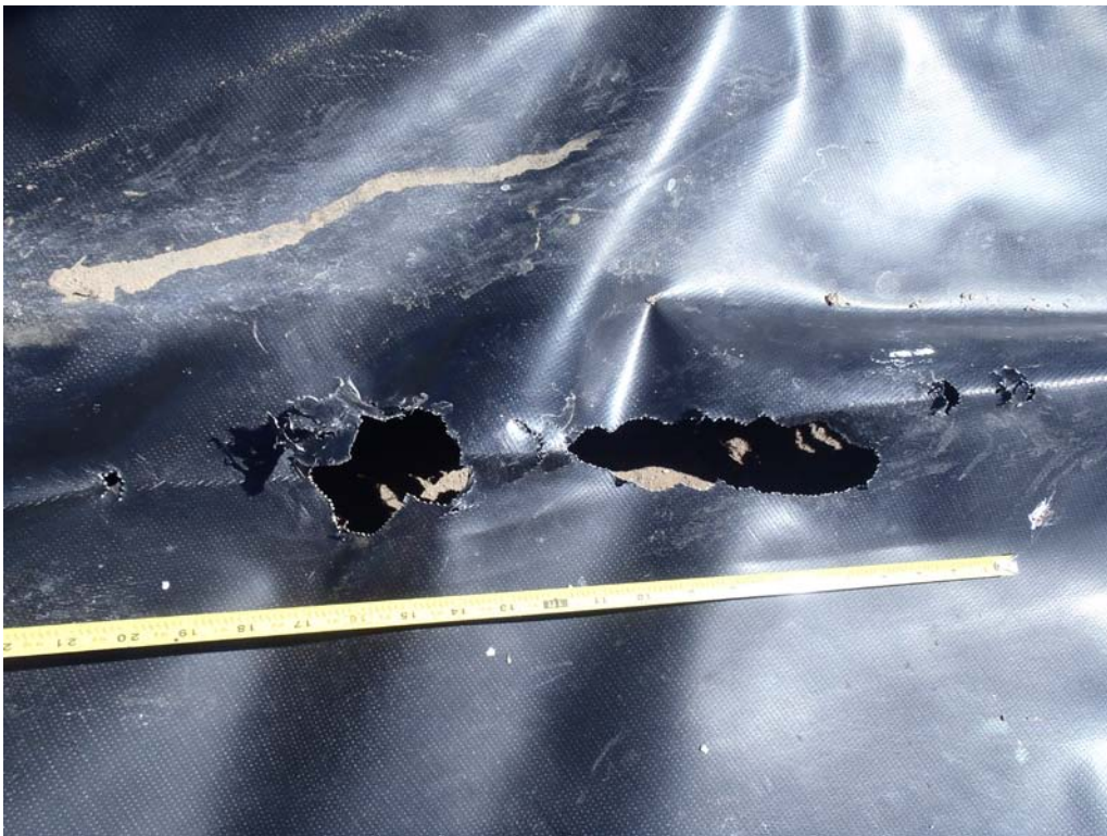
Xenon Upper Pit – Rodent damage.
