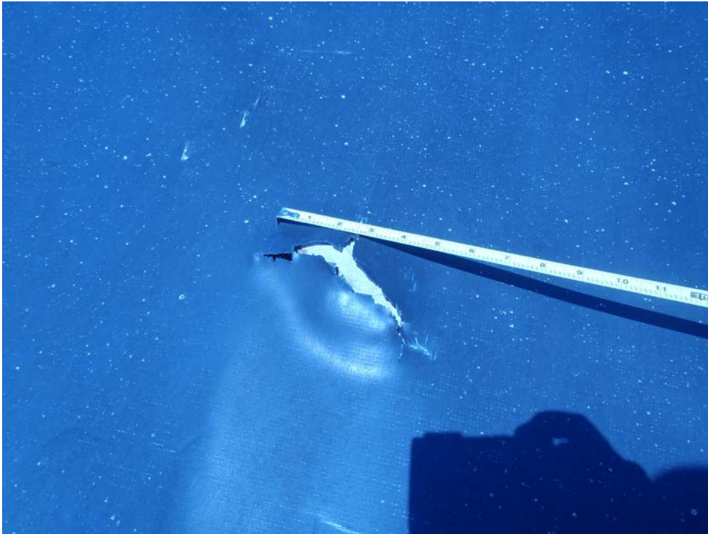
Xenon Middle Pit – Complete rock protrusion.
