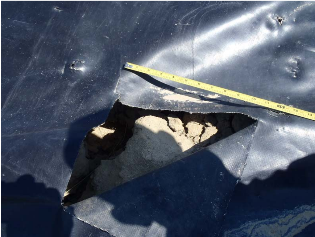
Xenon Upper Pit – Complete rock protrusion.
