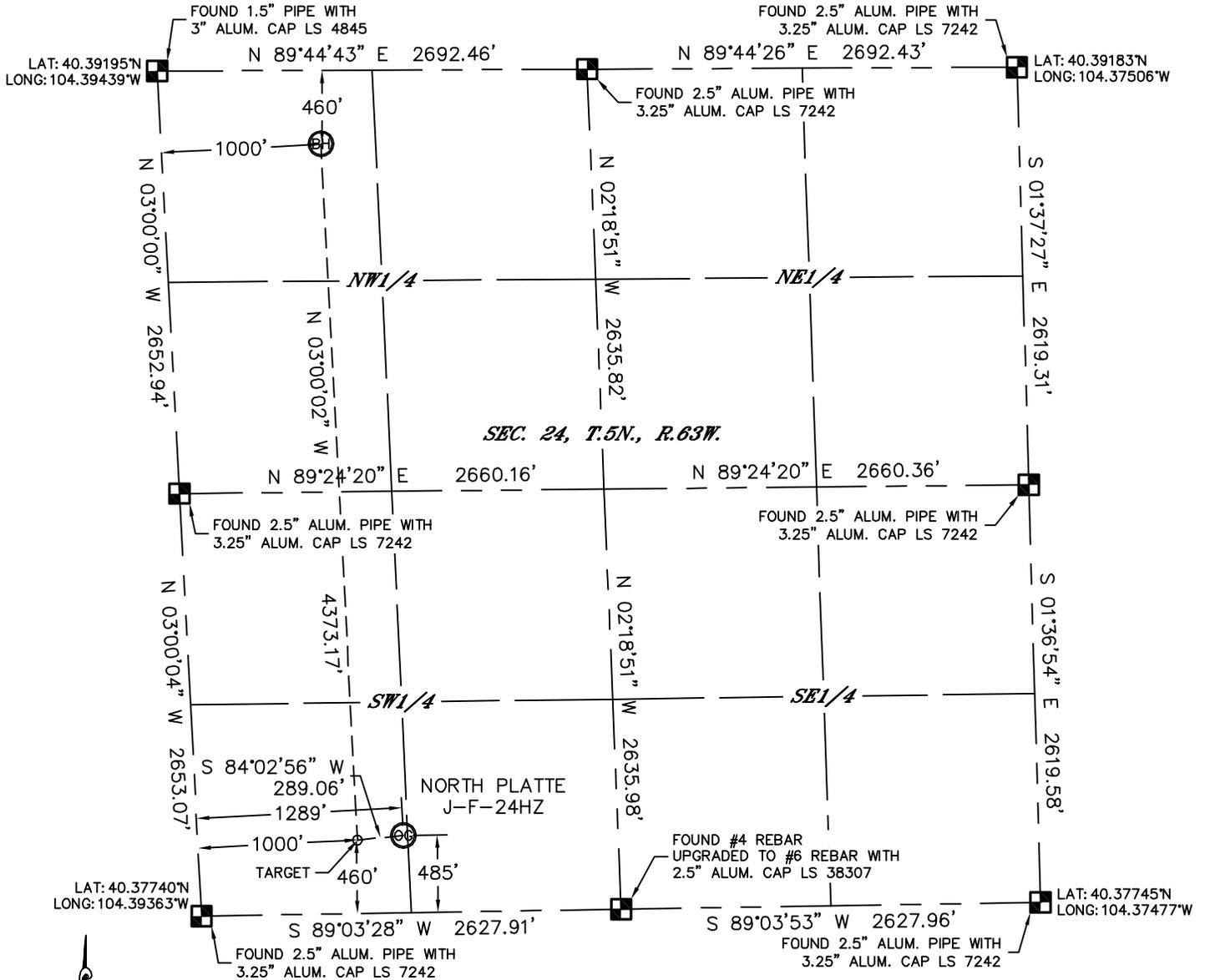
In accordance with a request from Keith Caplan with BONANZA CREEK ENERGY, INC. Lat40°, Inc. has determined the surface location of the NORTH PLATTE J-F-24HZ to be 485' from the SOUTH line and 1289' from the WEST line and the bottom hole to be 460' from the NORTH line and 1000' from the WEST line as measured at right angles from the section lines of Section 24, Township 5 North, Range 63 West of the Sixth Principal Meridian, County of Weld, State of Colorado.
