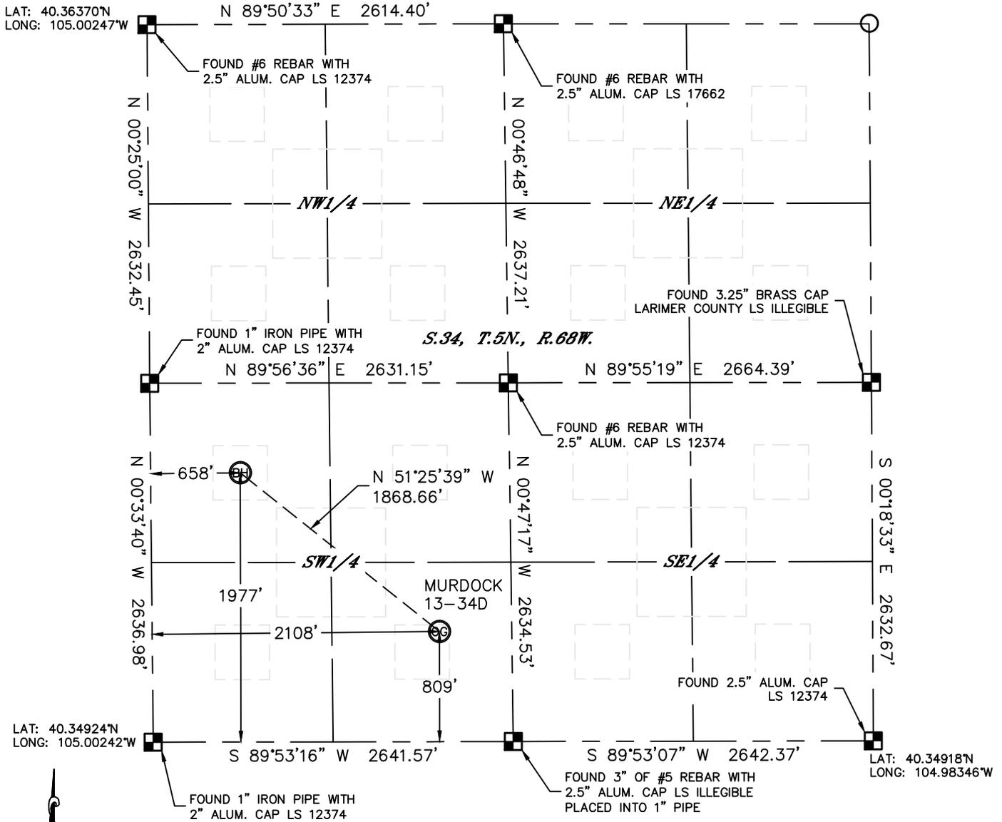
In accordance with a request from Jesse White with APOLLO OPERATING, LLC. Lat40°, Inc. has determined the surface location of the MURDOCK 13-34D to be 809' from the SOUTH line and 2108' from the WEST line and the bottom hole to be 1977' from the SOUTH line and 658' from the WEST line as measured at right angles from the section lines of Section 34, Township 5 North, Range 68 West of the Sixth Principal Meridian, County of Larimer, State of Colorado.
