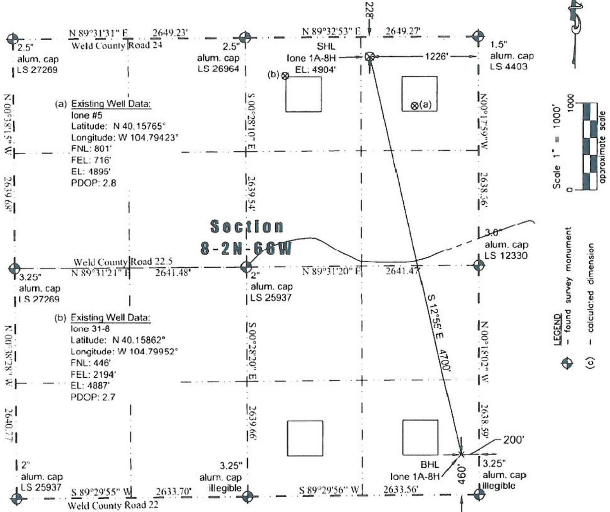
In accordance with a request from Jay Knutson of EnCana Oil & Gas (USA) Inc., JR Land Surveying, LLC has determined the location of the **lone 1A-8H** well site to be SHL: 228' FNL and 1226' FEL, (BHL 460' FSL and 200' FEL), as measured at ninety (90) degrees from the section lines of Section 8, Township 2 North, Range 66 West of the 6th Principal Meridian, Weld County Colorado.
