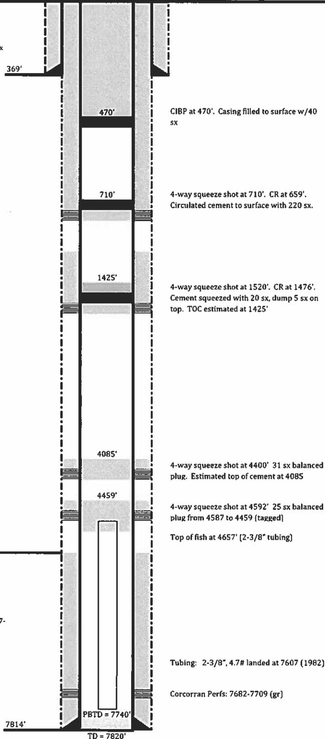
CIBP at 470'. Casing filled to surface w/40 sx
