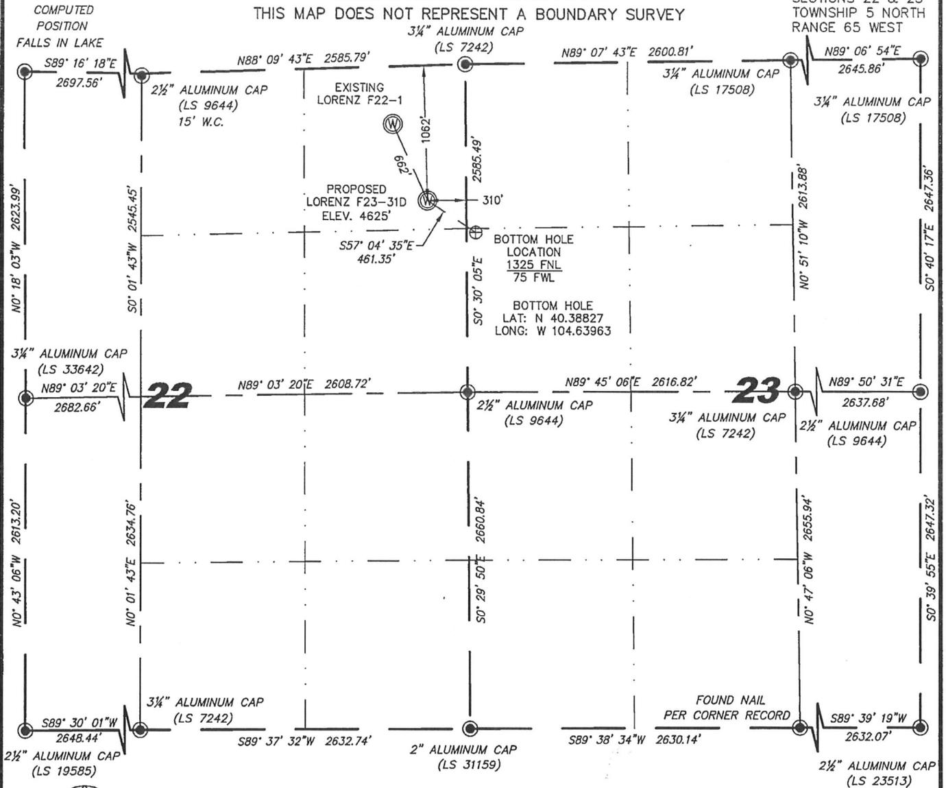
IN ACCORDANCE WITH A REQUEST FROM RYAN HAWKINS - NOBLE ENERGY INC, STEIL SURVEYING SERVICES, LLC HAS DETERMINED THE LOCATION OF THE LORENZ F23-31D WELL TO BE 1062' FNL, 310' FEL, AS MEASURED AT NINETY (90) DEGREES FROM THE SECTION LINES, SECTION 22, TOWNSHIP 5 NORTH, RANGE 65 WEST, 6TH PRINCIPLE MERIDIAN, WELD COUNTY, COLORADO.
