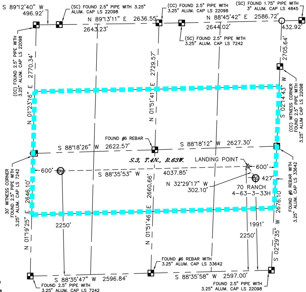
In accordance with a request from Glenn Berglund with BILL BARRETT CORPORATION Lat40°, Inc. has determined the surface location of the 70 RANCH 4-63-3-33H to be 1991' from the SOUTH line and 427' from the EAST line and the bottom hole to be 2250' from the SOUTH line and 600' from the WEST line as measured at right angles from the section lines of Section 3, Township 4 North, Range 63 West of the Sixth Principal Meridian, County of Weld, State of Colorado.
