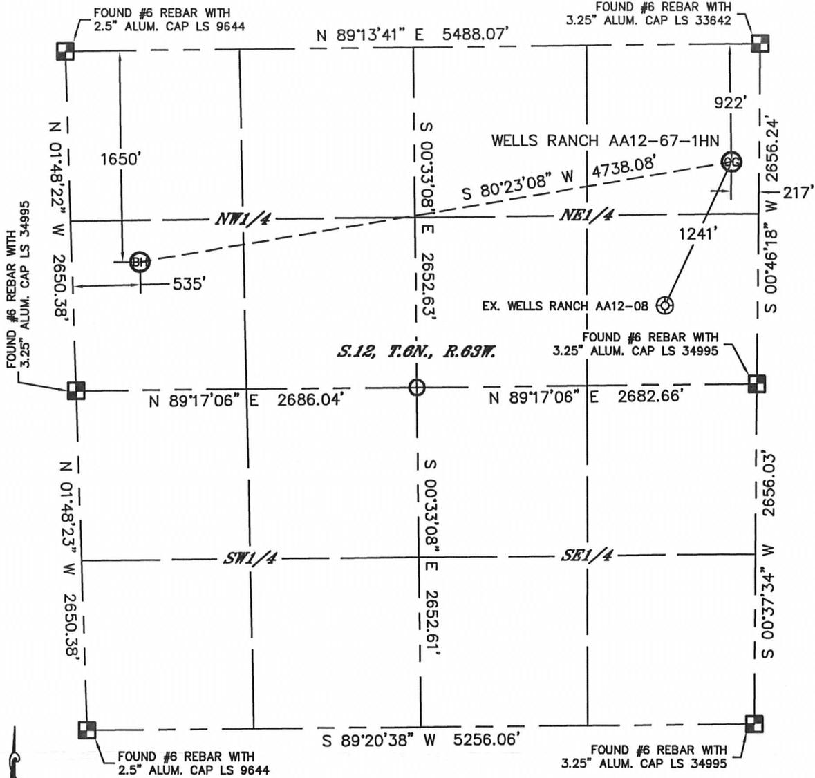
In accordance with a request from Sean Casper with Noble Energy Inc., Lat40°, Inc. has determined the surface location of the WELLS RANCH AA12-67-1HN to be 922' from the NORTH line and 217' from the EAST line and the bottom hole to be 1650' from the NORTH line and 535' from the WEST line as measured at right angles from the section lines of Section 12, Township 6 North, Range 63 West of the Sixth Principal Meridian, County of Weld, State of Colorado.
