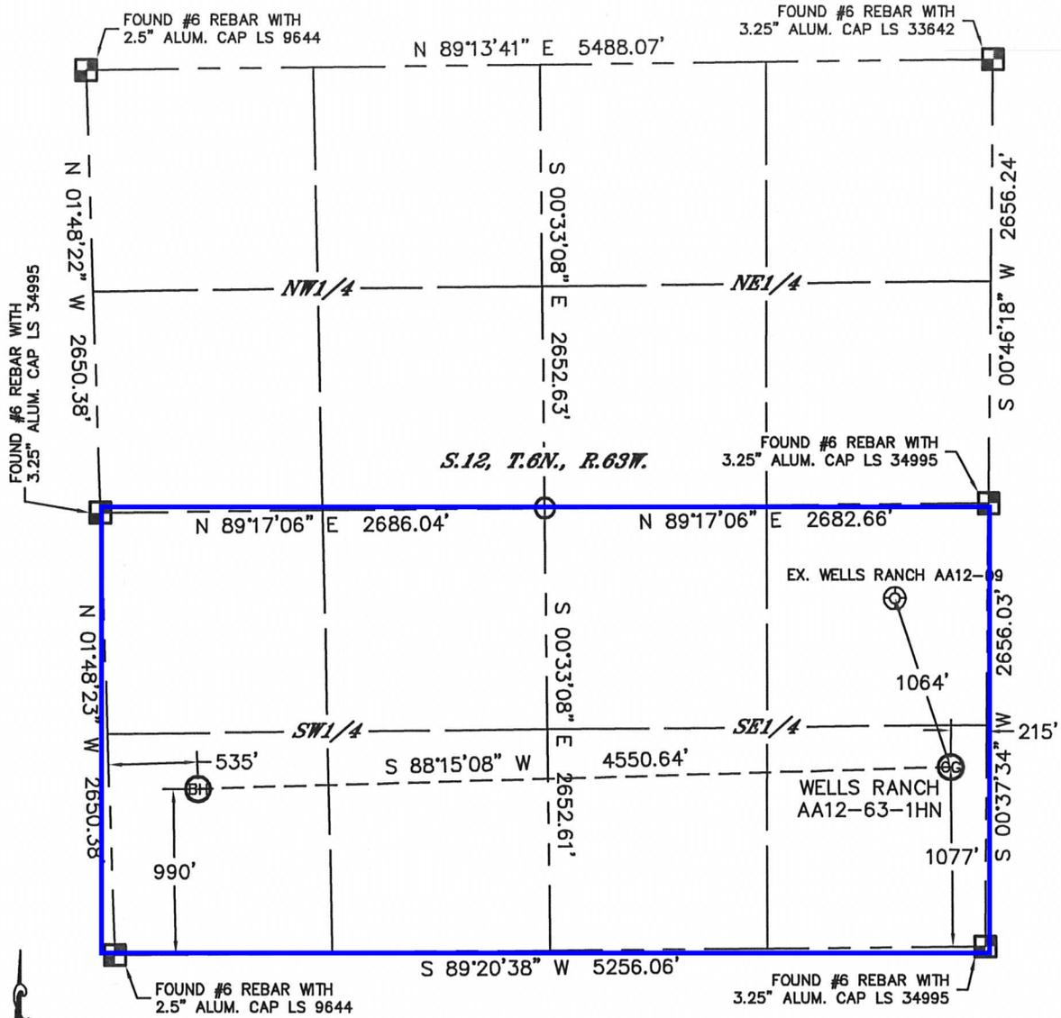
In accordance with a request from Sean Casper with Noble Energy Inc. Lat40°, Inc. has determined the surface location of the WELLS RANCH AA12-63-1HN to be 1077' from the SOUTH line and 215' from the EAST line and the bottom hole to be 990' from the SOUTH line and 535' from the WEST line as measured at right angles from the section lines of Section 12, Township 6 North, Range 63 West of the Sixth Principal Meridian, County of Weld, State of Colorado.
