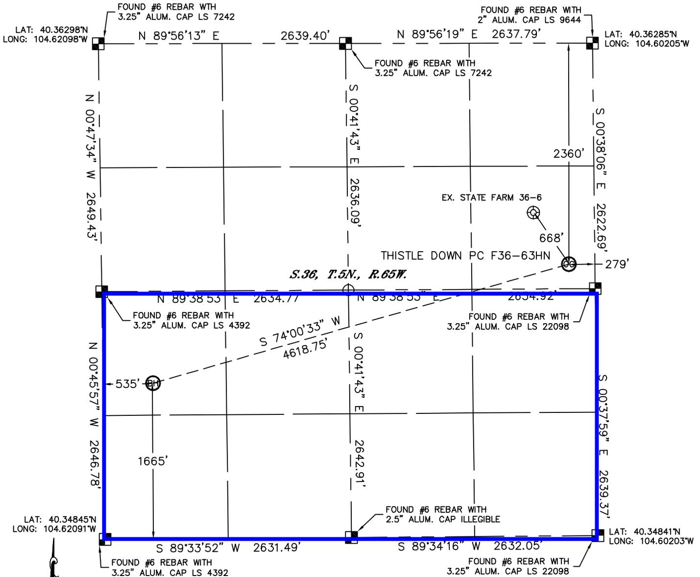
In accordance with a request from Jacob Rice with Noble Energy Inc., Lat40°, Inc. has determined the surface location of the THISTLE DOWN PC F36-63HN to be 2360' from the NORTH line and 279' from the EAST line and the bottom hole to be 1665' from the SOUTH line and 535' from the WEST line as measured at right angles from the section lines of Section 36, Township 5 North, Range 65 West of the Sixth Principal Meridian, County of Weld, State of Colorado.
