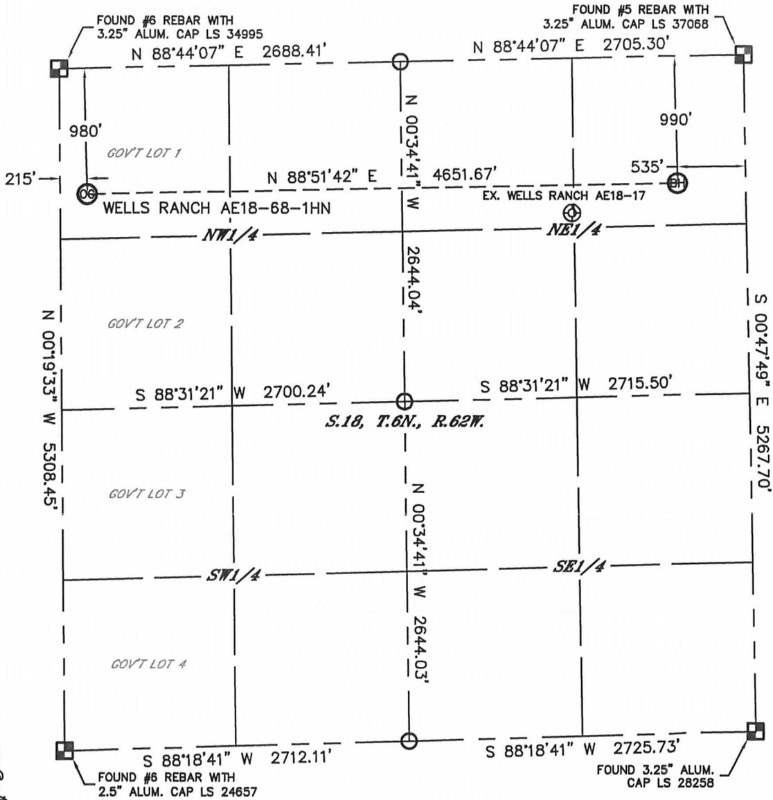
In accordance with a request from Sean Casper with Noble Energy Inc., Lat40°, Inc. has determined the surface location of the WELLS RANCH AE18-68-1HN to be 980' from the NORTH line and 215' from the WEST line and the bottom hole to be 990' from the NORTH line and 535' from the EAST line as measured at right angles from the section lines of Section 18, Township 6 North, Range 62 West of the Sixth Principal Meridian, County of Weld, State of Colorado.
