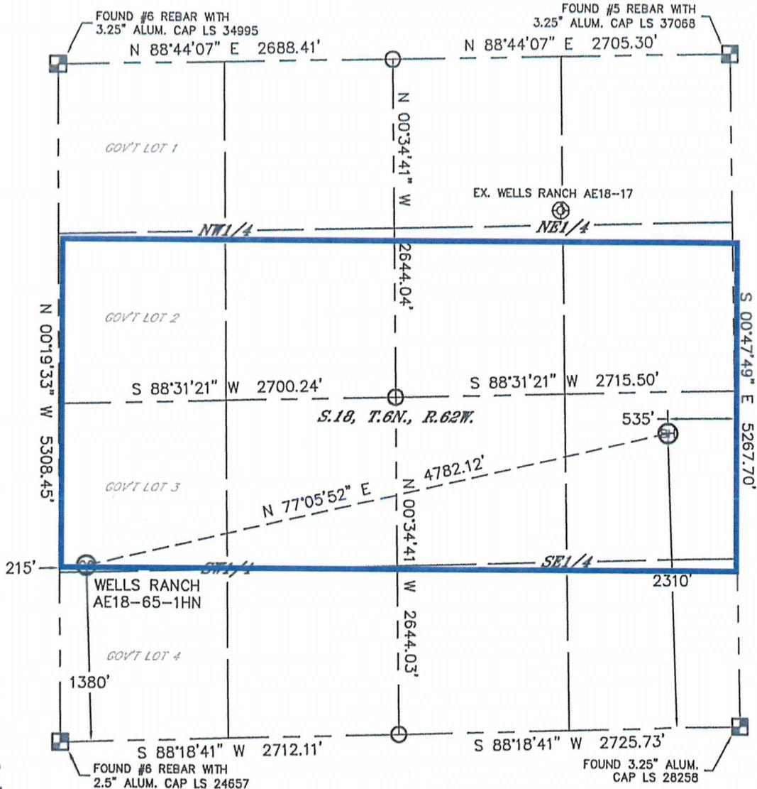
In accordance with a request from Sean Casper with Noble Energy Inc., Lat40°, Inc. has determined the surface location of the WELLS RANCH AE18-65-1HN to be 1380' from the SOUTH line and 215' from the WEST line and the bottom hole to be 2310' from the SOUTH line and 535' from the EAST line as measured at right angles from the section lines of Section 18, Township 6 North, Range 62 West of the Sixth Principal Meridian, County of Weld, State of Colorado.
