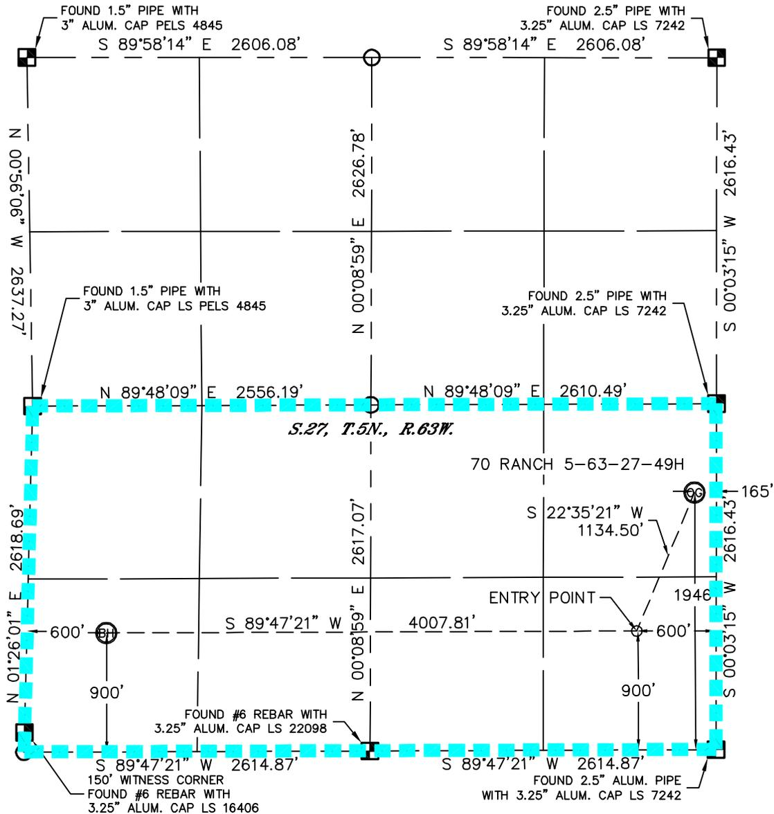
In accordance with a request from Glenn Berglund with BILL BARRETT CORPORATION Lat40°, Inc. has determined the surface location of the 70 RANCH 5-63-27-49H to be 1946' from the SOUTH line and 165' from the EAST line and the bottom hole to be 900' from the SOUTH line and 600' from the WEST line as measured at right angles from the section lines of Section 27, Township 5 North, Range 63 West of the Sixth Principal Meridian, County of Weld, State of Colorado.
