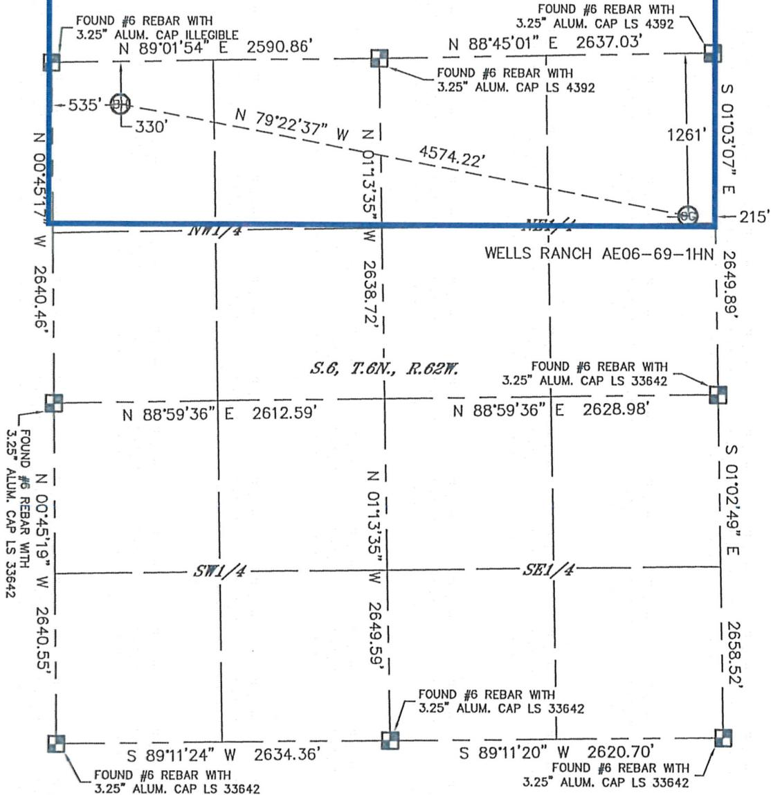
In accordance with a request from Sean Casper with Noble Energy Inc. Lat40°, Inc. has determined the surface location of the WELLS RANCH AE06-69-1HN to be 1261' from the NORTH line and 215' from the EAST line and the bottom hole to be 330' from the NORTH line and 535' from the WEST line as measured at right angles from the section lines of Section 6, Township 6 North, Range 62 West of the Sixth Principal Meridian, County of Weld, State of Colorado.
