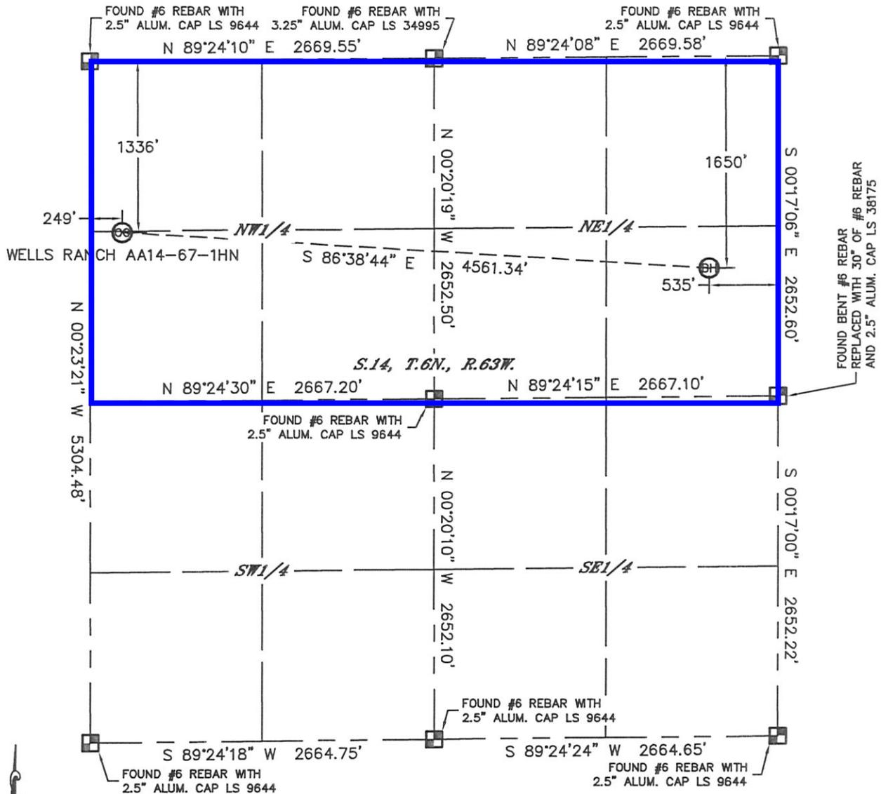
In accordance with a request from Sean Casper with Noble Energy Inc. Lat40°, Inc. has determined the surface location of the WELLS RANCH AA14-67-1HN to be 1336' from the NORTH line and 249' from the WEST line and the bottom hole to be 1650' from the NORTH line and 535' from the EAST line as measured at right angles from the section lines of Section 14, Township 6 North, Range 63 West of the Sixth Principal Meridian, County of Weld, State of Colorado.
