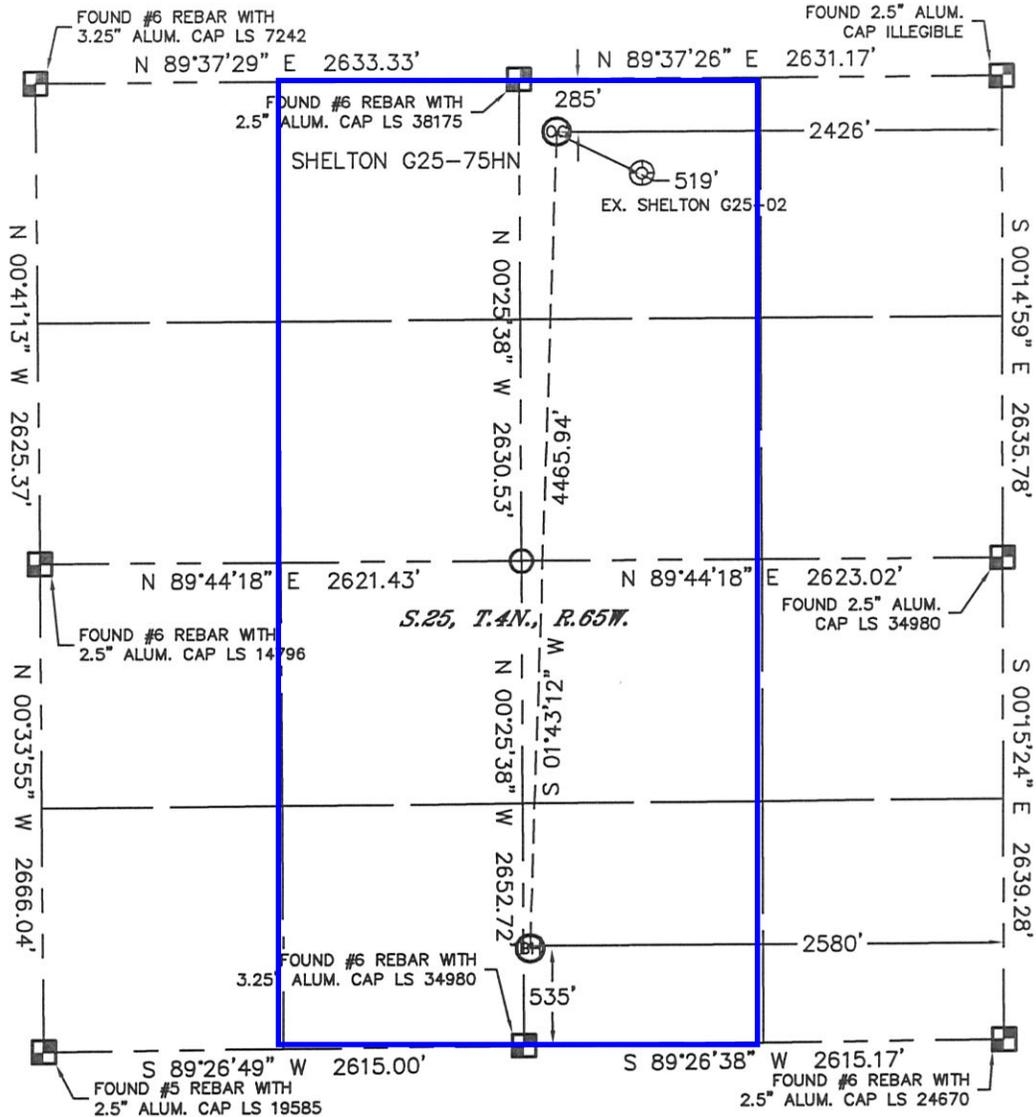
In accordance with a request from Ryan Hawkins with Noble Energy Inc., Lat40°, Inc. has determined the surface location of the SHELTON G25-75HN to be 285' from the NORTH line and 2426' from the EAST line and the bottom hole to be 535' from the SOUTH line and 2580' from the EAST line as measured at right angles from the section lines of Section 25, Township 4 North, Range 65 West of the Sixth Principal Meridian, County of Weld, State of Colorado.
