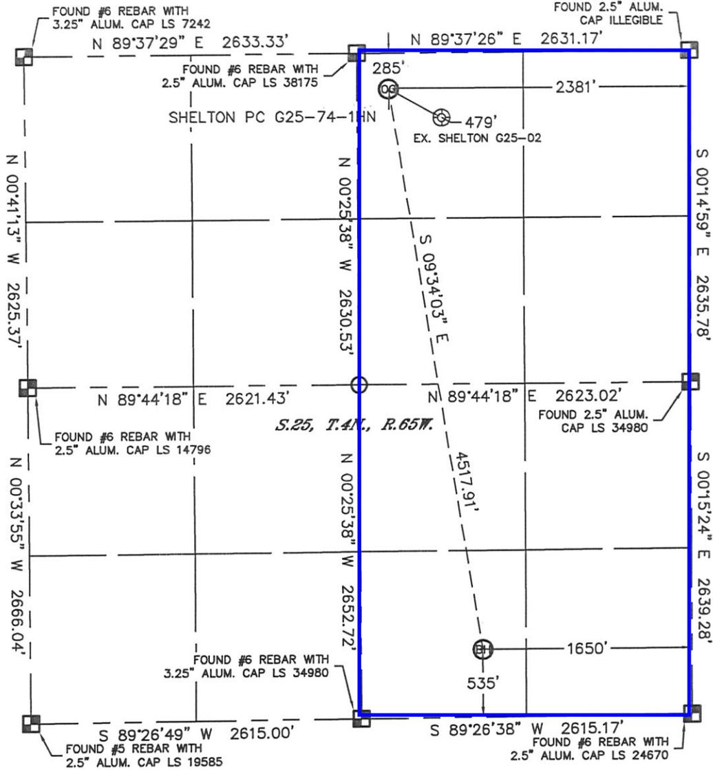
In accordance with a request from Ryan Hawkins with Noble Energy Inc. Lat40°, Inc. has determined the surface location of the SHELTON PC G25-74-1HN to be 285' from the NORTH line and 2381' from the EAST line and the bottom hole to be 535' from the SOUTH line and 1650' from the EAST line as measured at right angles from the section lines of Section 25, Township 4 North, Range 65 West of the Sixth Principal Meridian, County of Weld, State of Colorado.
