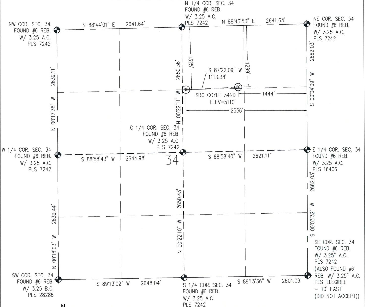
IN ACCORDANCE WITH A REQUEST FROM CRAIG RASMUSON - SYNERGY RESOURCES, BASELINE ENGINEERING CORP. HAS DETERMINED THE LOCATION OF THE SRC COYLE 34ND TO BE 1,299' FNL AND 1,444' FEL, AS MEASURED AT NINETY (90) DEGREES FROM THE SECTION LINE OF SECTION 34, TOWNSHIP 4 NORTH, RANGE 68 WEST AND THE BOTTOM HOLE LOCATION TO BE 1,325' FNL AND 2,556' FEL OF SECTION 34, TOWNSHIP 4 NORTH, RANGE 68 WEST, 6TH PRINCIPAL MERIDIAN, WELD COUNTY, COLORADO.
