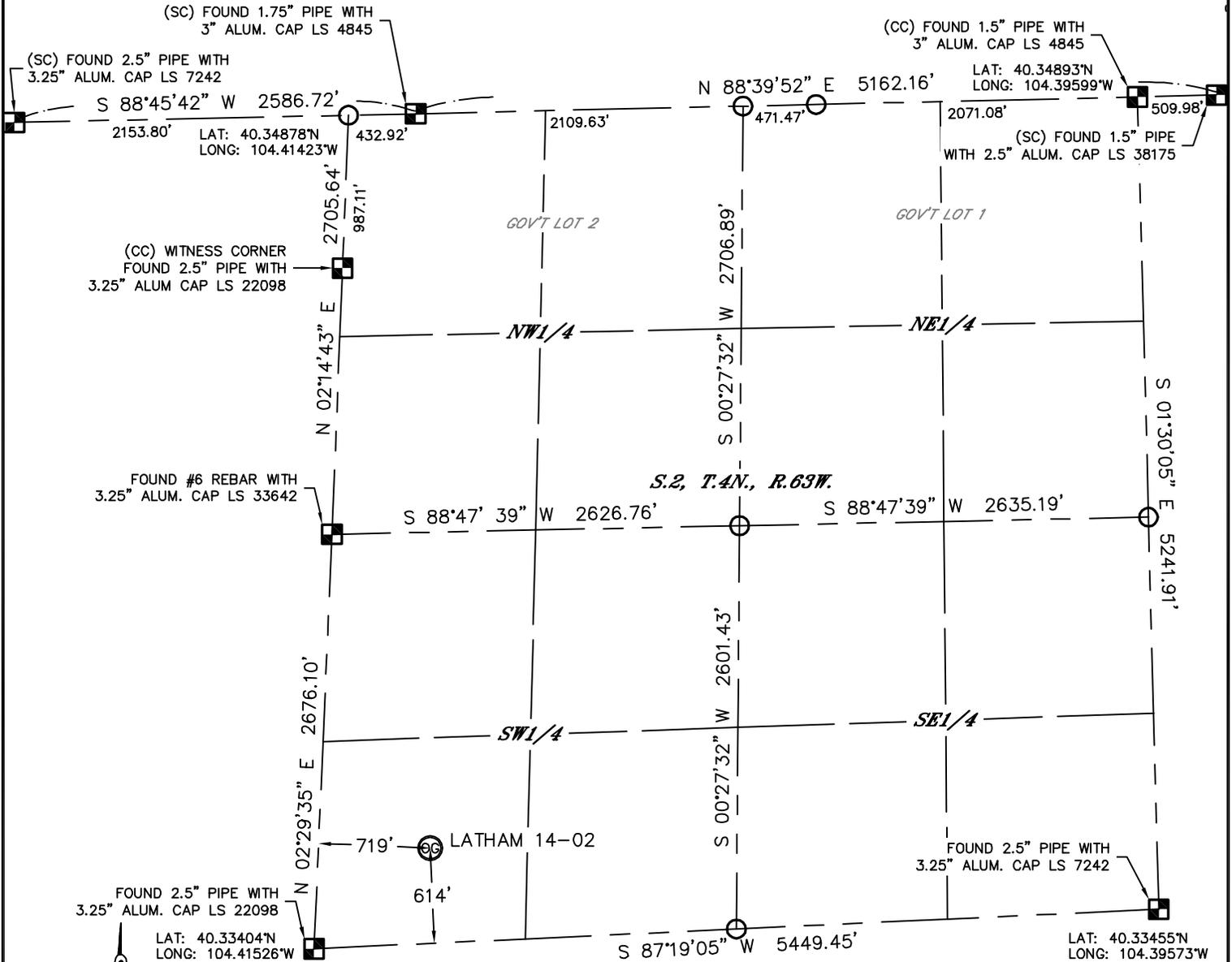
In accordance with a request from Keith Caplan with BONANZA CREEK ENERGY, INC. Lat40°, Inc. has determined the surface location of the LATHAM 14-02 to be 614' from the SOUTH line and 719' from the WEST line as measured at right angles from the section lines of Section 2, Township 4 North, Range 63 West of the Sixth Principal Meridian, County of Weld, State of Colorado.
