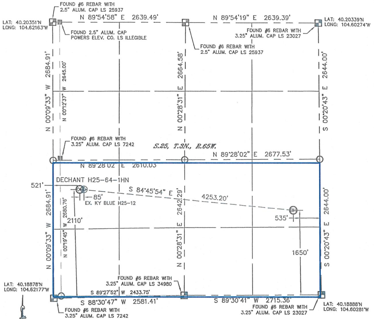
In accordance with a request from Mike Rodine with Noble Energy Inc. Lat40°, Inc. has determined the surface location of the DECHANT H25-64-1HN to be 2110' from the SOUTH line and 521' from the WEST line and the bottom hole to be 1650' from the SOUTH line and 535' from the EAST line as measured at right angles from the section lines of Section 25, Township 3 North, Range 65 West of the Sixth Principal Meridian, County of Weld, State of Colorado.
