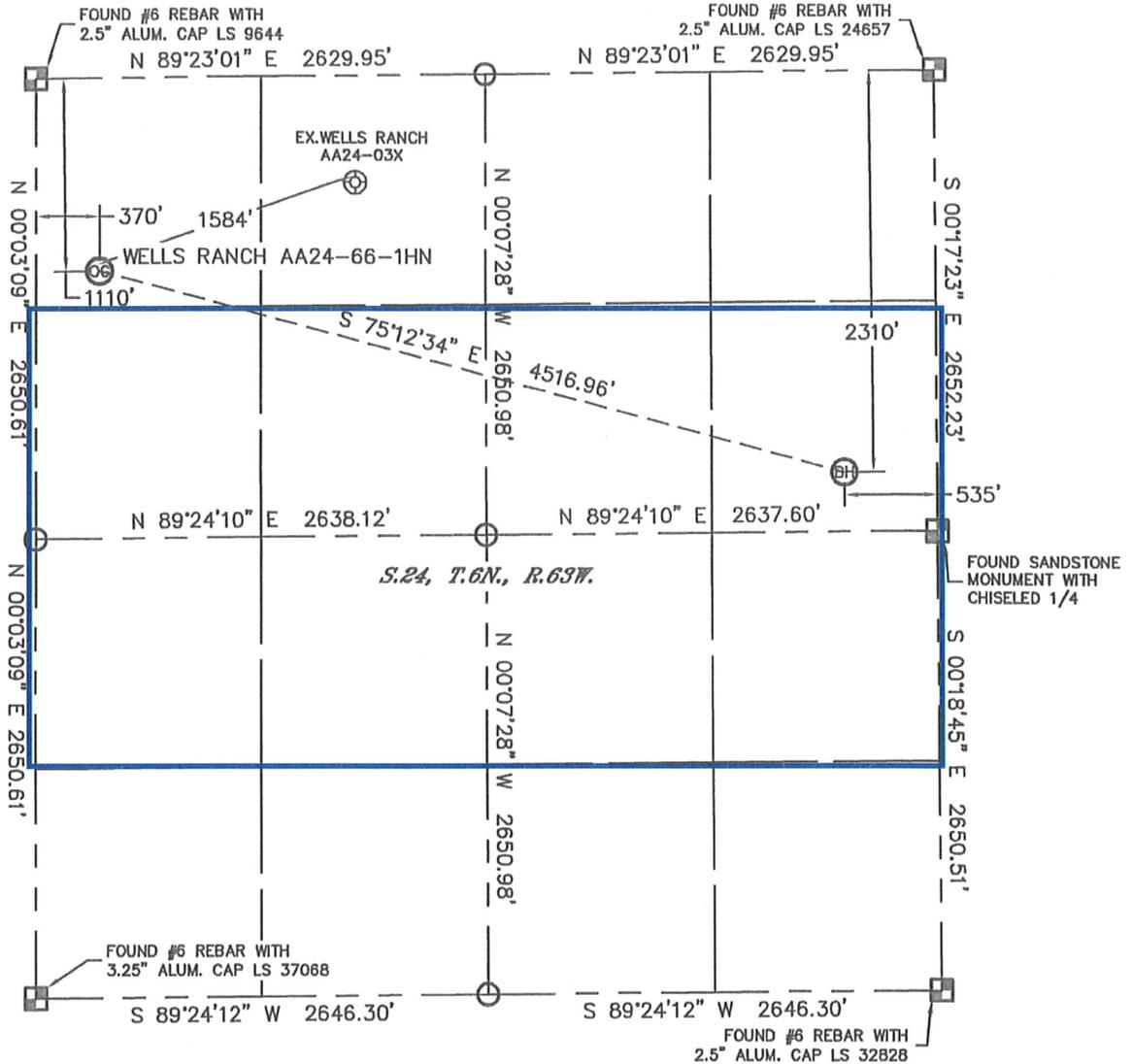
In accordance with a request from Sean Casper with Noble Energy Inc., Lat40°, Inc. has determined the surface location of the WELLS RANCH AA24-66-1HN to be 1110' from the NORTH line and 370' from the WEST line and the bottom hole to be 2310' from the NORTH line and 535' from the EAST line as measured at right angles from the section lines of Section 24, Township 6 North, Range 63 West of the Sixth Principal Meridian, County of Weld, State of Colorado.
