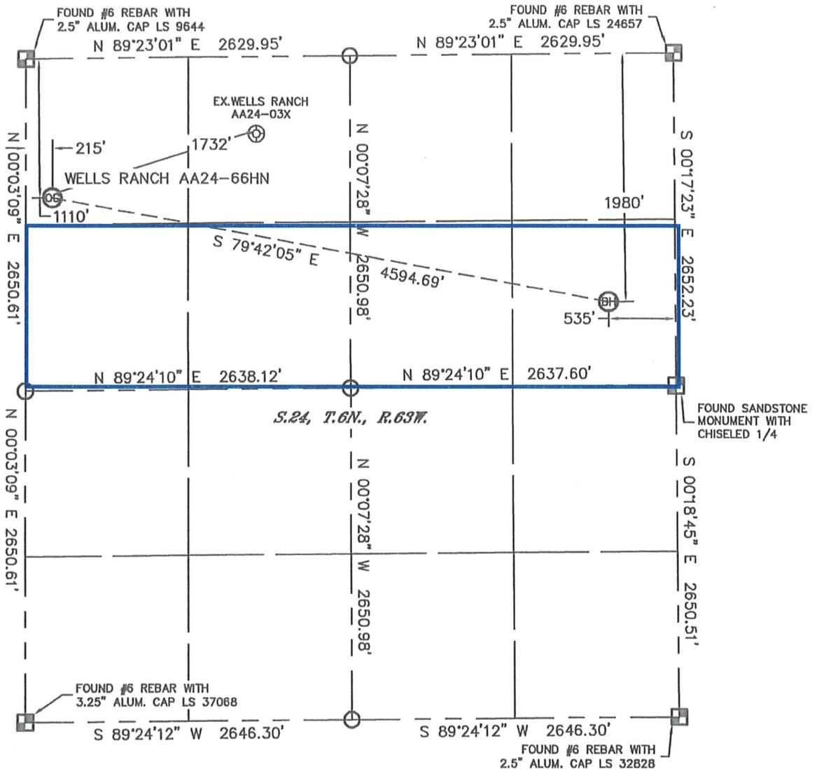
In accordance with a request from Sean Casper with Noble Energy Inc. Lat40°, Inc. has determined the surface location of the WELLS RANCH AA24-66HN to be 1110' from the NORTH line and 215' from the WEST line and the bottom hole to be 1980' from the NORTH line and 535' from the EAST line as measured at right angles from the section lines of Section 24, Township 6 North, Range 63 West of the Sixth Principal Meridian, County of Weld, State of Colorado.
