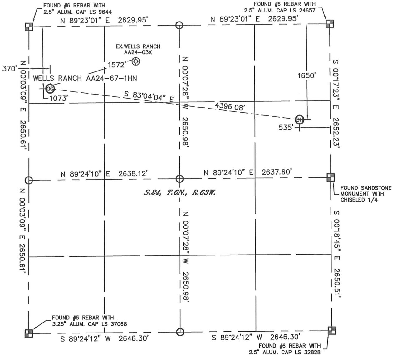
In accordance with a request from Sean Casper with Noble Energy Inc. Lat40°, Inc. has determined the surface location of the WELLS RANCH AA24-67-1HN to be 1073' from the NORTH line and 370' from the WEST line and the bottom hole to be 1650' from the NORTH line and 535' from the EAST line as measured at right angles from the section lines of Section 24, Township 6 North, Range 63 West of the Sixth Principal Meridian, County of Weld, State of Colorado.
