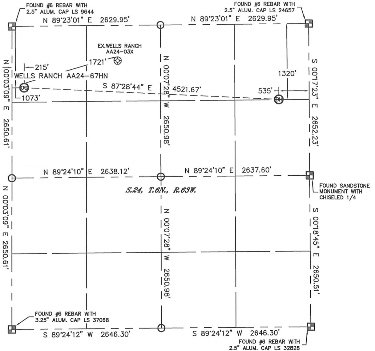
In accordance with a request from Sean Casper with Noble Energy Inc. Lat40°, Inc. has determined the surface location of the WELLS RANCH AA24-67HN to be 1073' from the NORTH line and 215' from the WEST line and the bottom hole to be 1320' from the NORTH line and 535' from the EAST line as measured at right angles from the section lines of Section 24, Township 6 North, Range 63 West of the Sixth Principal Meridian, County of Weld, State of Colorado.
