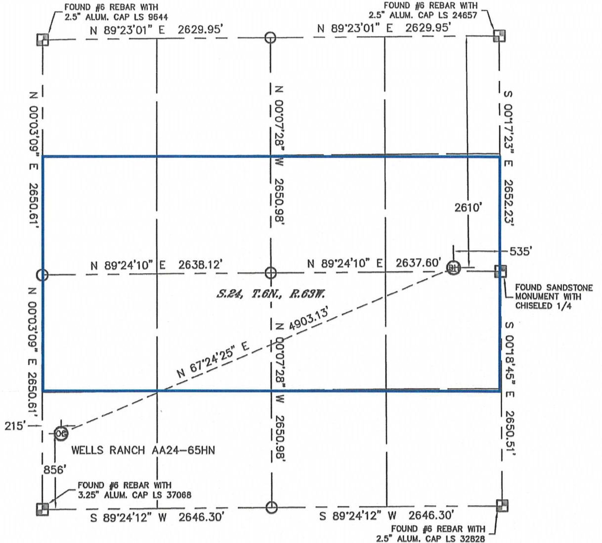
In accordance with a request from Sean Casper with Noble Energy Inc. Lat40°, Inc. has determined the surface location of the WELLS RANCH AA24-65HN to be 856' from the SOUTH line and 215' from the WEST line and the bottom hole to be 2610' from the NORTH line and 535' from the EAST line as measured at right angles from the section lines of Section 24, Township 6 North, Range 63 West of the Sixth Principal Meridian, County of Weld, State of Colorado.
