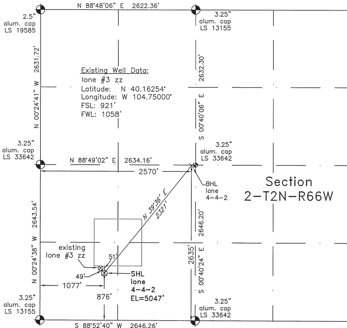
In accordance with a request from Dave Bale of EnCana Oil & Gas (USA) Inc., Frederick Land Surveying, Inc. has determined the location of the **lone 4-4-2** well site to be SHL: 876' FSL and 1077' FWL, BHL (2635' FSL and 2570' FWL) as measured at ninety (90) degrees from the section lines of Section 2, Township 2 North, Range 66 West, 6th Principal Meridian, Weld County, CO.
