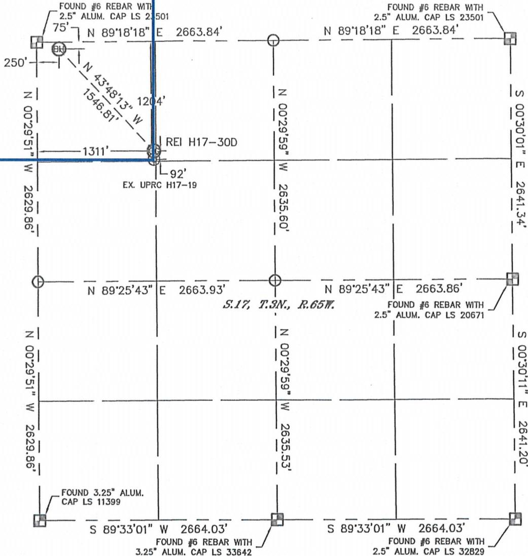
In accordance with a request from MIKE RODINE with Noble Energy Inc., Lat40°, Inc. has determined the surface location of the REI H17-30D to be 1204' from the NORTH line and 1311' from the WEST line and the bottom hole to be 75' from the NORTH line and 250' from the WEST line as measured at right angles from the section lines of Section 17, Township 3 North, Range 65 West of the Sixth Principal Meridian, County of Weld, State of Colorado.
