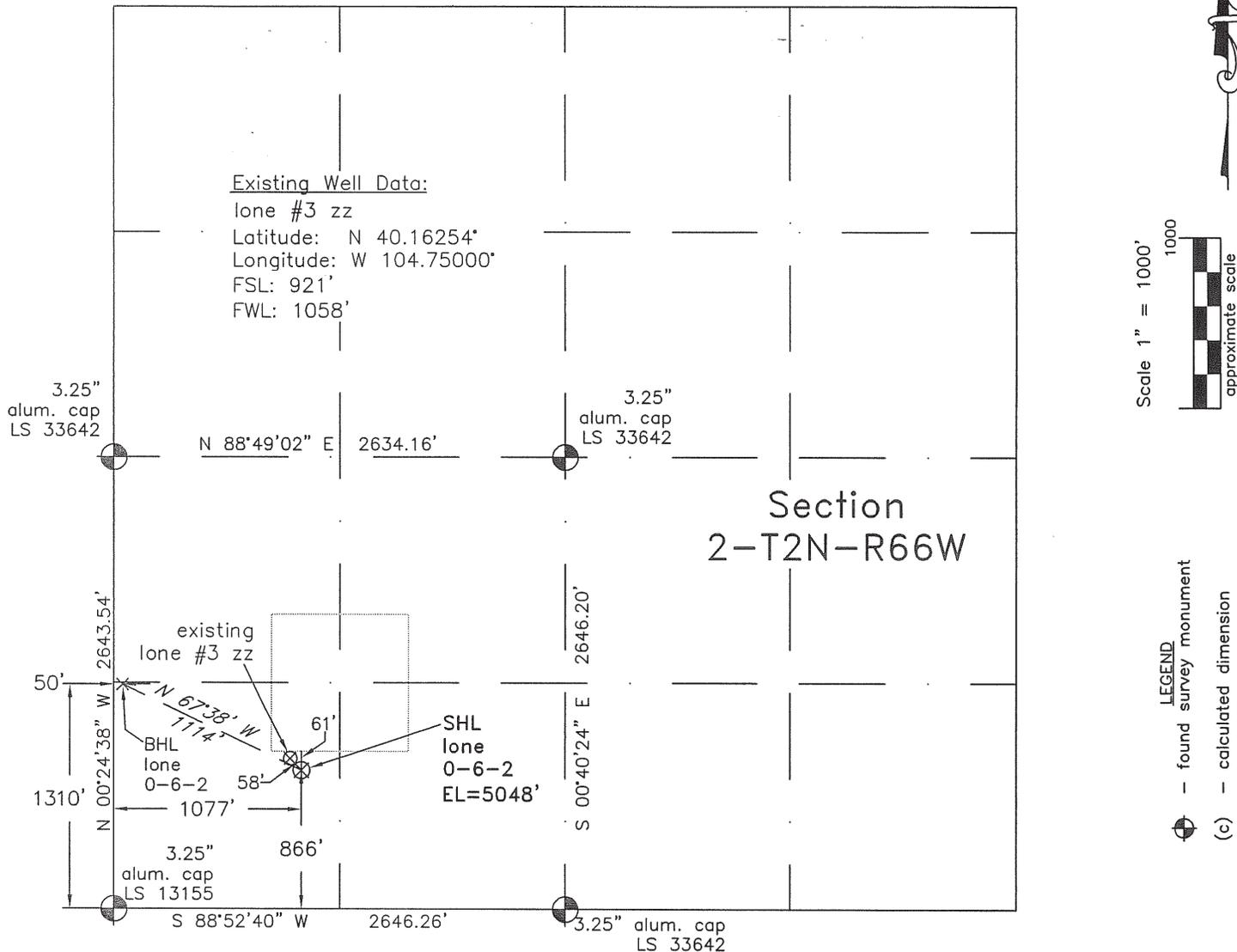
In accordance with a request from Dave Bale of EnCana Oil & Gas (USA) Inc., Frederick Land Surveying, Inc. has determined the location of the **lone 0-6-2** well site to be SHL: 866' FSL and 1077' FWL, BHL (1310' FSL and 50' FWL) as measured at ninety (90) degrees from the section lines of Section 2, Township 2 North, Range 66 West, 6th Principal Meridian, Weld County, CO.
