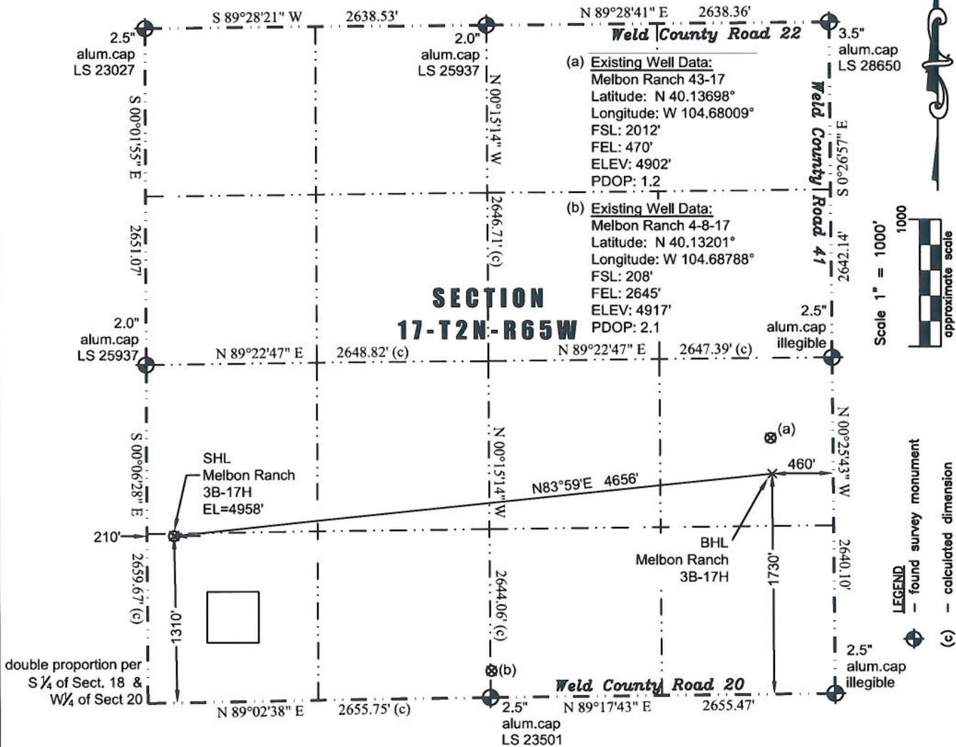
In accordance with a request from Jay Knutson of EnCana Oil & Gas (USA) Inc., JR Land Surveying, LLC has determined the location of the **Melbon Ranch 3B-17H** well site to be SHL: 1310' FSL and 210' FWL, (BHL 1730' FSL and 460' FEL), as measured at ninety (90) degrees from the section lines of Section 17, Township 2 North, Range 65 West of the 6th Principal Meridian, Weld County Colorado.
