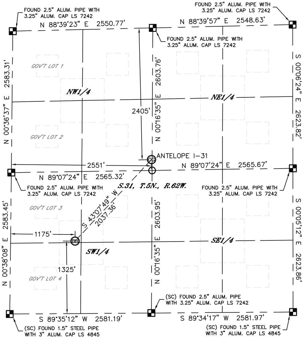
In accordance with a request from Keith Caplan with BONANZA CREEK ENERGY, INC. Lat40°, Inc. has determined the surface location of the ANTELOPE I-31 to be 2405' from the NORTH line and 2551' from the WEST line and the bottom hole to be 1325' from the SOUTH line and 1175' from the WEST line as measured at right angles from the section lines of Section 31, Township 5 North, Range 62 West of the Sixth Principal Meridian, County of Weld, State of Colorado.
