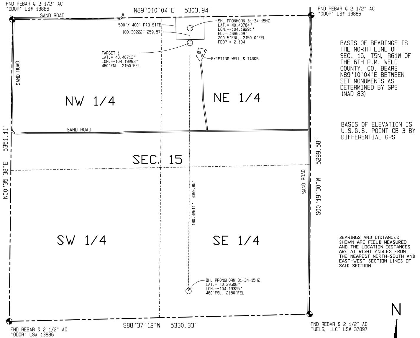
BASIS OF BEARINGS IS THE NORTH LINE OF SEC. 15, T5N, R61W OF THE 6TH P.M. WELD COUNTY, CO. BEARS N89°10'04"E BEARS SET MONUMENTS AS DETERMINED BY GPS (NAD 83)
